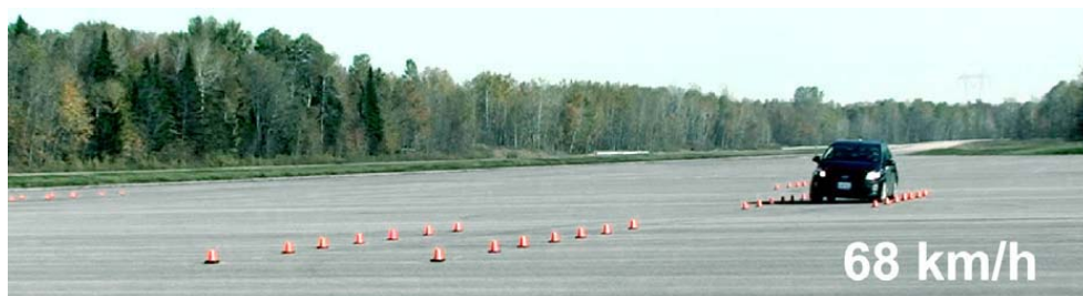
Figure 9: 2010 Toyota Prius during emergency lane change manoeuvre test
