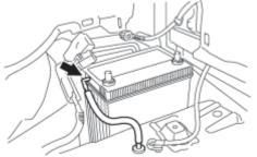
(b) Connect the battery ventilation hose to the battery without kinking it.
