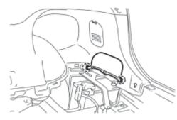
(a) Disengage the 2 claws and remove the No. 3 rear floor board plate upper.
