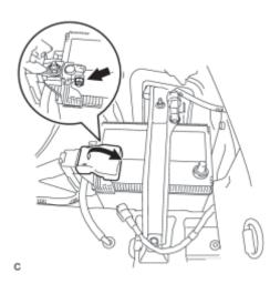
(e) Connect the positive (+) battery terminal with the nut.
