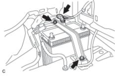
(c) Install the battery clamp with the bolt and nut.
