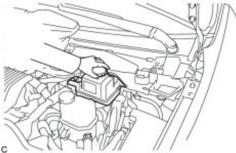
(1) Remove the brake master cylinder reservoir filler cap assembly.
