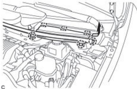
(1) Slide the hood to cowl top seal and disengage the claw.
