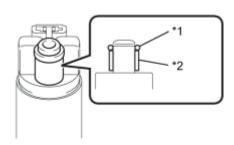
(a) Apply gasoline to a new O-ring. Then install the O-ring and spacer to the fuel pump.
