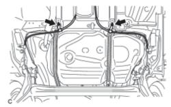
(a) Remove the 2 bolts and disconnect the parking brake cable assembly.
