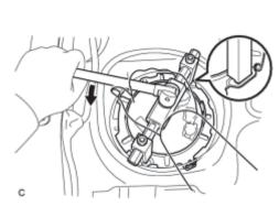
• Loosen the retainer by turning it counterclockwise while holding SST down. Do not allow the claw of the tank suction tube support to slip out of its groove on the fuel tank.
