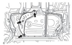
(a) Remove the 3 bolts and the No. 1 fuel tank protector.
