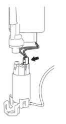
(f) Disconnect the fuel pump harness connector.
