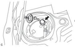
(c) Disconnect the fuel pump connector.
