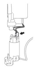
(b) Connect the fuel pump harness connector.
