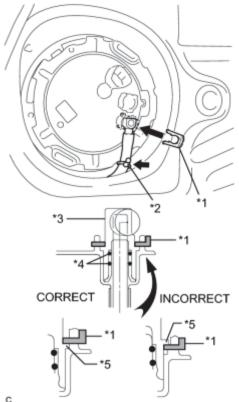
(a) Push the fuel tube joint in the plug of the fuel suction plate, then install the tube joint clip.
