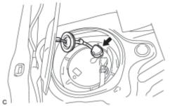
(b) Connect the fuel pump connector.
