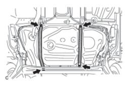
(c) Tighten the 4 set bolts of the 2 fuel tank bands.
