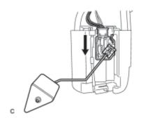
(a) Install the fuel sender gauge assembly by sliding it downward.
