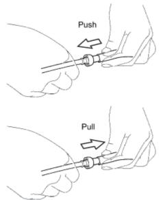
(2) Match the axis of the connector with the axis of the pipe, and push the pipe into the connector until the connector makes a "click" sound. If the pipe is difficult to push into the connector, apply a small amount of clean engine oil to the tip of the pipe.
