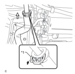
(a) Push in the hose connector to the filler pipe and install the retainer.
