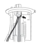
(a) Disconnect the connector of the fuel pump harness.
