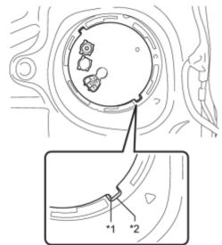
(b) Install the fuel suction tube assembly with pump and gauge to the fuel tank.
