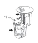
(a) Do not disconnect the tube shown in the illustration when disassembling the fuel suction tube assembly with pump and gauge. Doing so will cause reassembly of the fuel suction tube assembly with pump and gauge to be impossible as the tube is welded to the plate.
