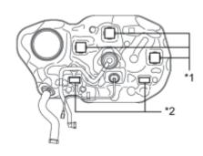
(a) Install 3 new No. 1 fuel tank cushions and 2 new No. 2 fuel tank cushions as shown in the illustration.
