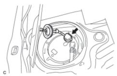
(b) Disconnect the fuel pump connector.
