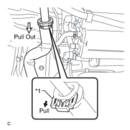
(b) Pull out the fuel tank to filler pipe hose.
