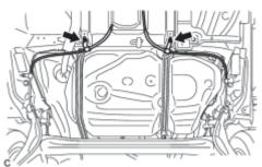
(d) Connect the parking brake cable assembly with the 2 bolts.
