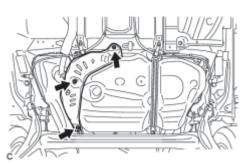
(a) Install the No. 1 fuel tank protector with the 3 bolts.
