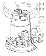
(e) Using a screwdriver with its tip wrapped in protective tape, disengage the 5 claws, and remove the fuel pump filter and fuel pump from the fuel filter.
