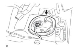
(a) Remove the rear floor service hole cover.
