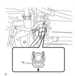
(a) Push in the fuel cut-off tube connector to the charcoal canister and push up the retainer so that the claws engage.
