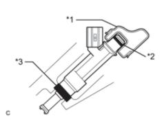
(b) Install the injector into the delivery pipe and cylinder head as shown in the illustration. Apply grease or gasoline to the contact surfaces of the injector before installing the injector.
