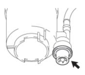
(a) Using a screwdriver with its tip wrapped in protective tape, remove the fuel pressure regulator assembly.
