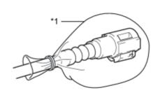
(5) Cover the disconnected pipe and connector with a plastic bag to prevent damage and contamination.
