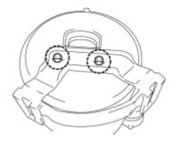
(d) Using a screwdriver with its tip wrapped in protective tape, disengage the 2 claws and remove the No. 1 fuel suction support.
