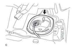
(b) Remove the rear floor service hole cover.
