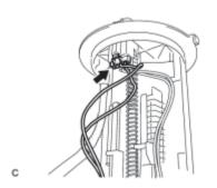
(b) Connect the connector of the fuel sender gauge assembly.
