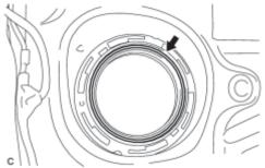
(b) Remove the gasket from the fuel tank.
