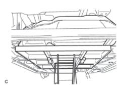
(b) Support the fuel tank using an engine lifter.
