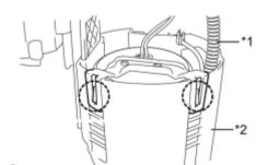
(c) Using a screwdriver with its tip wrapped in protective tape, disengage the 2 claws, and remove the fuel filter and fuel pump from the fuel subtank.
