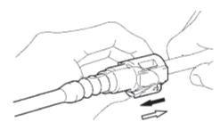
(3) If the connector and pipe are stuck, pinch the fuel pipe by hand and push or pull the connector to disconnect it.
