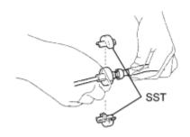
(4) Assemble SST to the connector as shown in the illustration.
