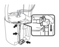
(f) Align the groove of the fuel pump filter hose with the cutout of the fuel sub-tank and install the hose.
