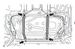
(c) Remove the 4 set bolts of the 2 fuel tank bands.
