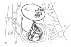
(a) Remove the fuel suction tube assembly with pump and gauge from the fuel tank.
