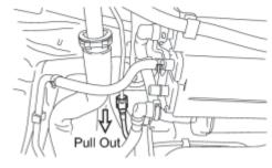
(a) Pinch the tabs of the retainer to remove the lock claws and pull it down as shown in the illustration.
