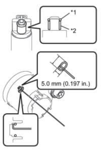
(g) Remove the O-ring and spacer from the fuel pump.
