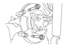
(b) Install the 2 rear disc brake pad guide pins to the rear disc brake cylinder mounting.
