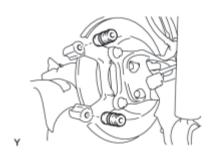
(b) Install the 2 rear disc brake bushing dust boots to the rear disc brake cylinder mounting.
