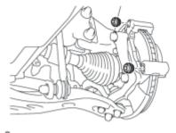
(b) Install the 2 front disc brake bushing dust boots to the front disc brake cylinder mounting.
