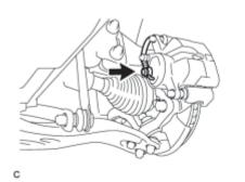
(a) Connect the front flexible hose to the disc brake cylinder assembly with a new union bolt and a new gasket.
