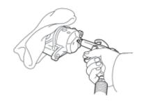
(a) Place a piece of cloth between the front disc brake piston and disc brake cylinder assembly.
