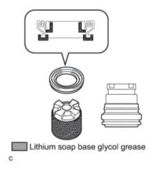
(b) Install the cylinder boot to the piston as shown in the illustration.
