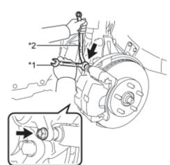
(a) Hold the front disc brake cylinder slide pin, and install the disc brake cylinder assembly to the front disc brake cylinder mounting with the 2 bolts.
