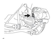
(a) Remove the union bolt and gasket, and separate the front flexible hose from the disc brake cylinder assembly.
