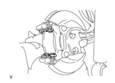
(a) Remove the 2 rear disc brake pad support plates from the disc brake cylinder mounting.
