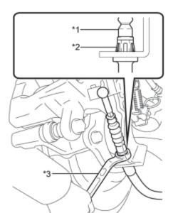
(b) Separate the No. 3 parking brake cable assembly from the rear disc brake cylinder assembly.
