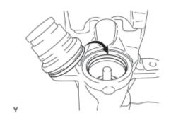
(a) Install the seal portion of the cylinder boot into the groove portion of the rear disc brake cylinder assembly.
