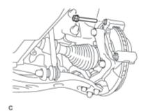
(b) Install the front No. 1 disc brake cylinder slide pin to the front disc brake cylinder mounting.
