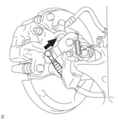
(a) Separate the No. 3 parking brake cable assembly from the rear disc brake cylinder assembly.
