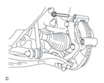
(a) Remove the front No. 1 disc brake cylinder slide pin from the front disc brake cylinder mounting.
