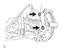
(a) Remove the 2 bolts and front disc brake cylinder mounting from the steering knuckle.
