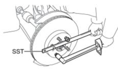
(b) Using SST to hold the disc, tighten the disc with the 5 nuts.
