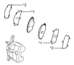
(a) Remove the front No. 1 anti-squeal shim and front No. 2 anti-squeal shim from each brake pad.
