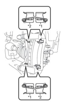
(a) Install the 2 front No. 1 disc brake pad support plates and 2 front No. 2 disc brake pad support plates to the front disc brake cylinder mounting.
