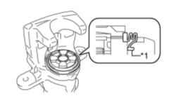
(d) Make sure that the cylinder boot is securely installed into the groove of the rear disc brake cylinder assembly and rear disc brake piston.
