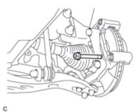
(b) Install the front No. 2 disc brake cylinder slide pin to the front disc brake cylinder mounting.
