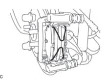
(a) Remove the 2 anti-squeal springs from the rear disc brake pads.
