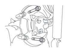
(a) Remove the 2 rear disc brake pad guide pins from the rear disc brake cylinder mounting.
