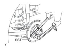
(b) While holding the disc using SST, tighten the disc with the 5 hub nuts.
