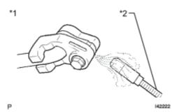
(c) Using a halogen leak detector, inspect for refrigerant leaks from the refrigerant lines.
