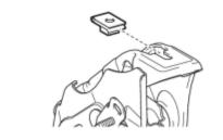
(a) Install the nut to the brake pedal support assembly.
