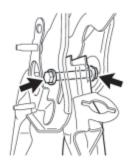
(a) Remove the brake pedal shaft and nut to remove the brake pedal sub-assembly from the brake pedal support sub-assembly.
