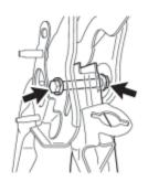
(a) Install the brake pedal sub-assembly to the brake pedal support subassembly with the brake pedal shaft and nut.
