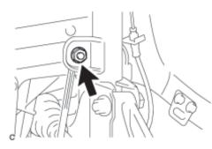
(a) Install the front stabilizer link assembly to the front shock absorber with coil spring with the nut.
