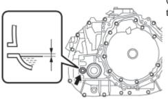
(a) Check that the fluid level is between 0 to 10 mm (0 to 0.394 in.) from the lowest position of the inner surface of the transaxle filler plug opening.
