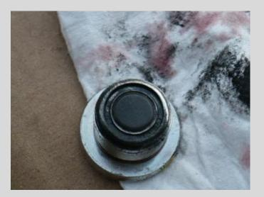
Remove Fill Plug the rest of the way Now. Attach Transfer Pump To One Quart At A Time, Place Transfer Pump Hose In Fill Opening And Pump New Fluid Into Transaxle.
