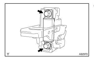
(b) Remove the 2 bolts and electric vehicle fuse.
