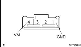
(17) Measure the voltage between the terminals on the blower motor connector.
