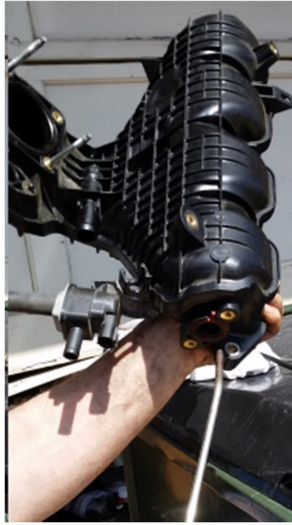
Cleaning Carbon Deposits with Air Nozzle
