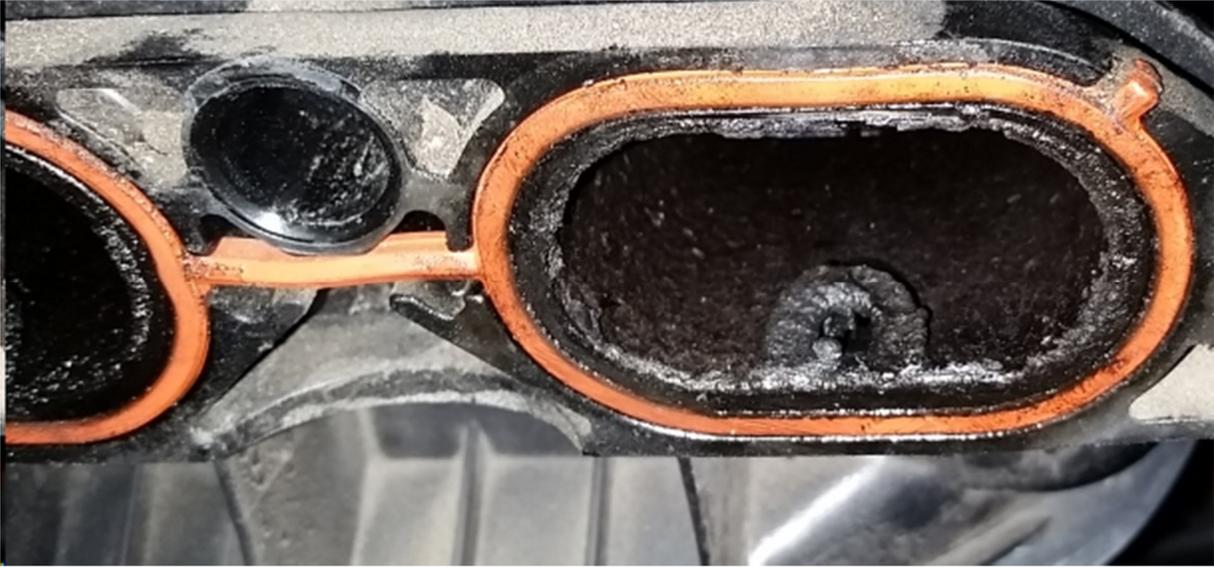
Carbon deposits clogging intake manifold (Prius.2)
