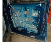
This is the surface to which the trim panel is attached. To the extent that it has resonant areas, add some CLD Tile. You will seldom need more than 1 or 2, cut into smaller pieces. This where I want to hang the barrier layers. There are two significant advantages to inner door skin barrier placement in most vehicles:
