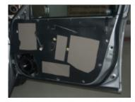
I add closed cell foam to the side of the MLV facing the trim panel where it will help decouple and stabilize the trim panel. This is less important if I will be lining the trim panel with 3M Thinsulate™ Acoustic.
