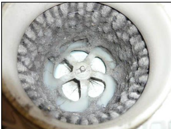
Figure 1. HV Battery Cooling Fan BEFORE Cleaning
