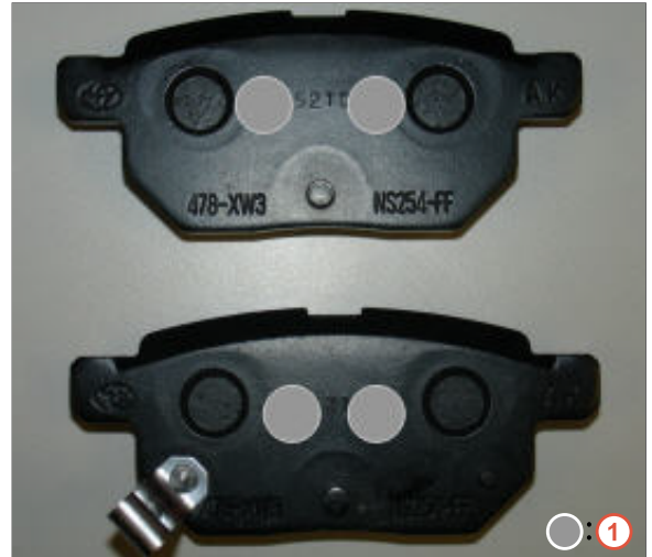
1 Grease Application Area
