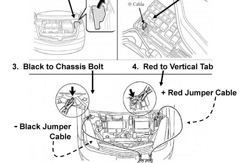
The 12V Auxiliary battery may be jump started if the vehicle does not start and the instrument cluster gauges are dim or off after depressing the brake pedal and pushing the power button.
