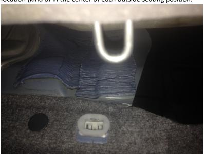
c. Access panel is glued down so I used a flat blade screwdriver to pry it up.
