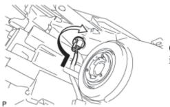
(b) Turn the clearance light bulb and headlight cord in the direction indicated by the arrow shown in the illustration and install them as a unit.
