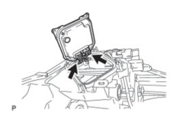
(b) Disconnect the 2 connectors and remove the headlight light control ECU sub-assembly.
