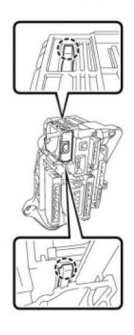
(a) Engage the 2 claws to install the tire pressure warning ECU.
