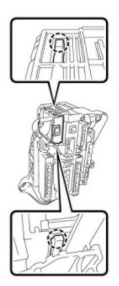
(a) Disengage the 2 claws to remove the tire pressure warning ECU.
