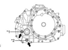
(a) Using a 10 mm hexagon socket wrench, remove the filler plug and gasket.
