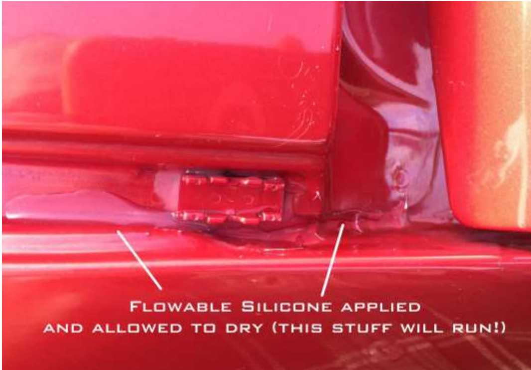
Photo #4 Close-up of the rear driver side roof gutter where suspect crack was
