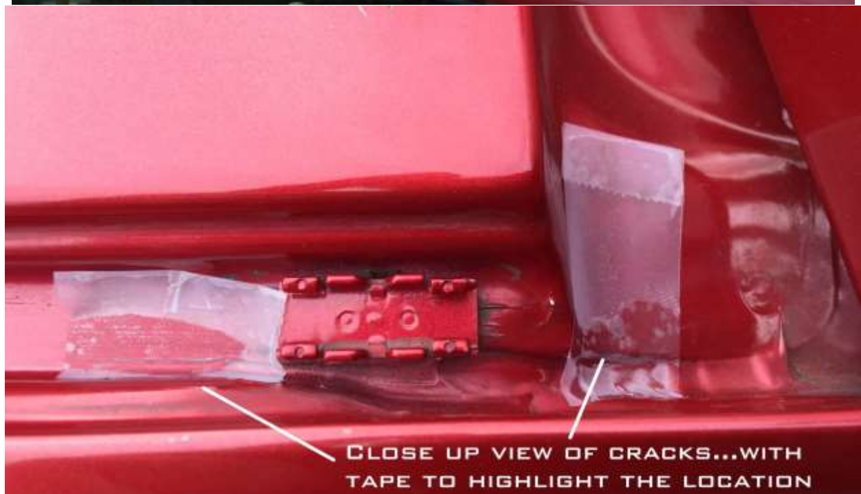
Photos #2 and #3 showing 'possible' crack and how SMALL the crack is...
