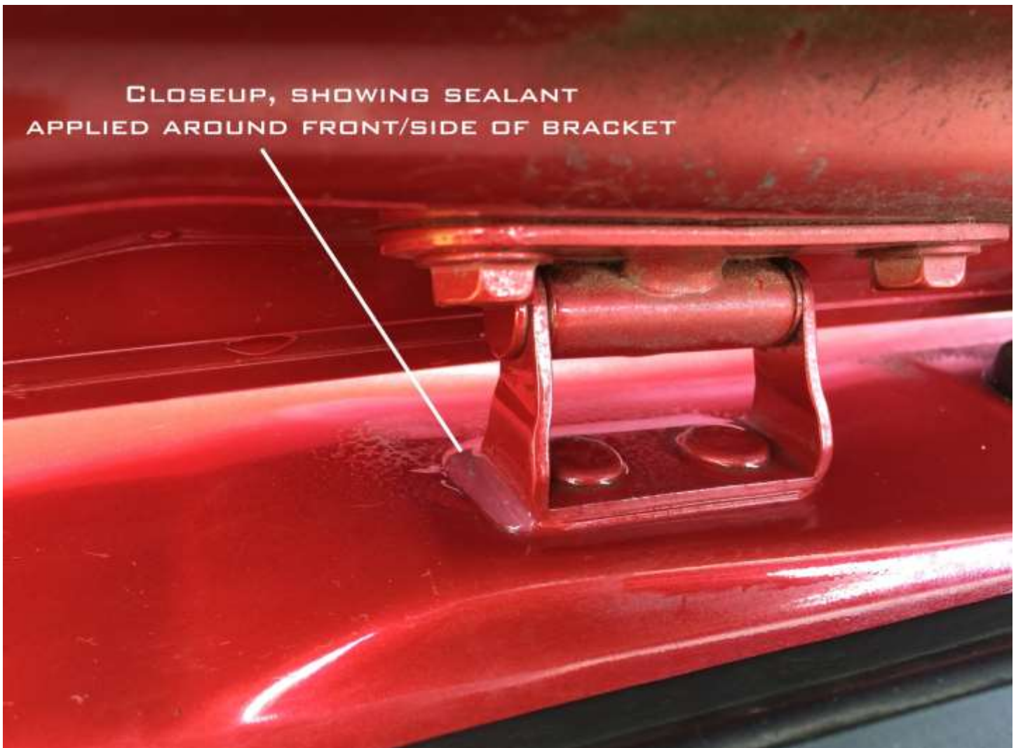
Photo #6 showing sealed hinge base where water could pool...note the checkered paint here...
