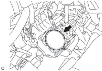
(a) Install a new gasket onto the intake manifold.
