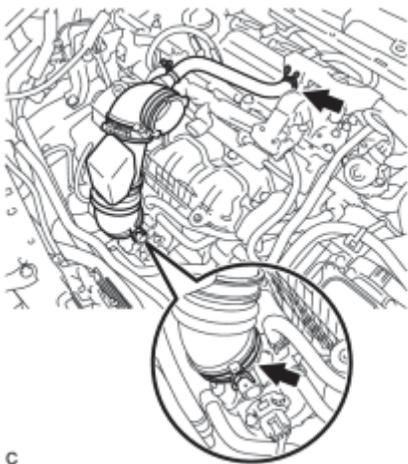
(a) Install the air cleaner hose assembly and lock the hose clamp.
