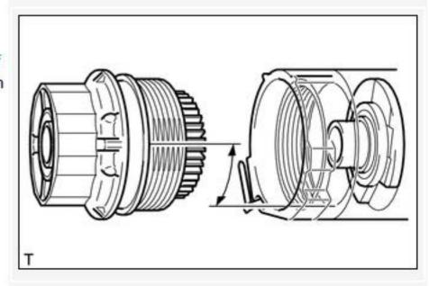
(f) Using SST, tighten the oil filter cap assembly.
