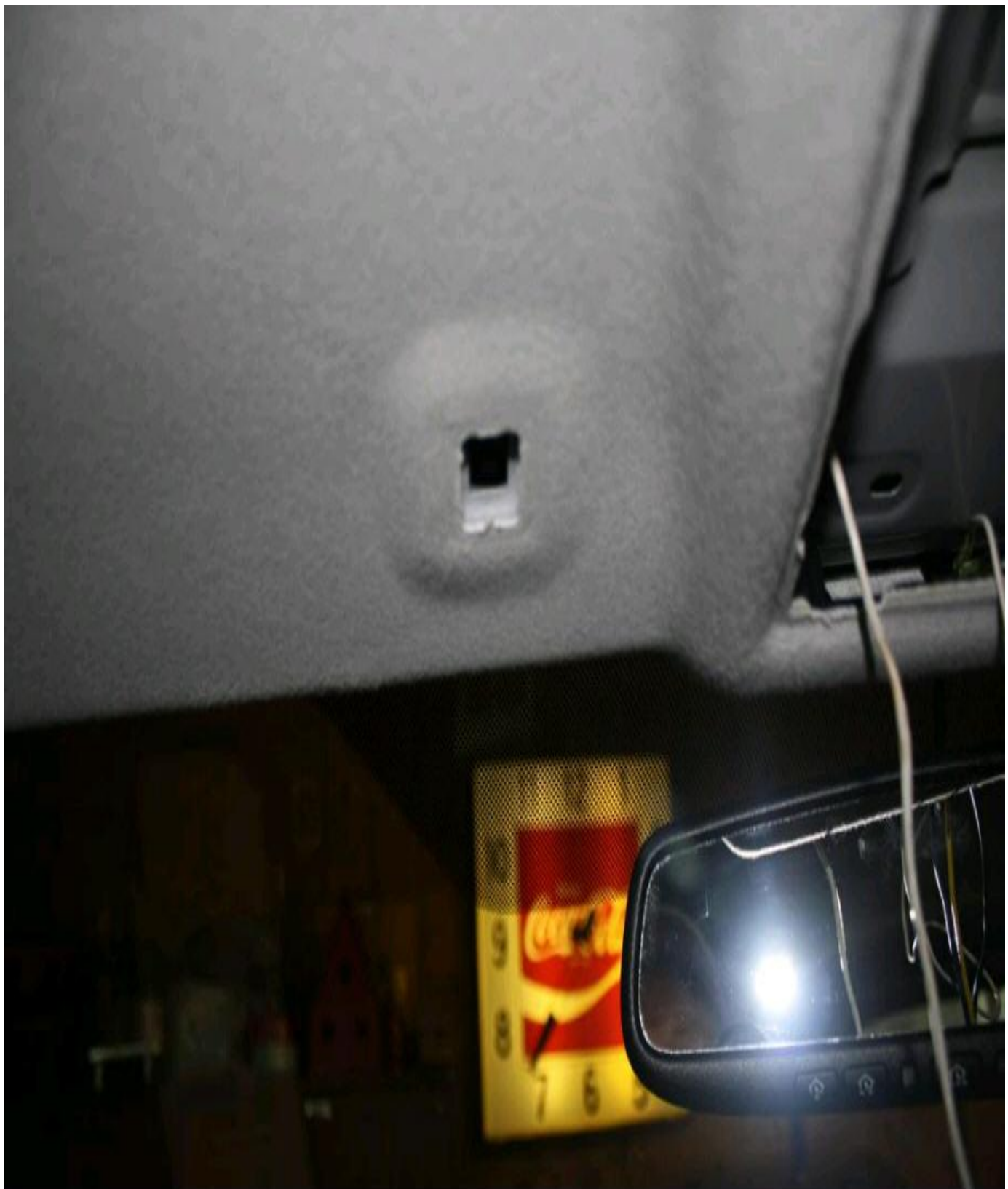
Sun Visor holder. Removes by turning counter clockwise. Once removed press clips on base to remove.
