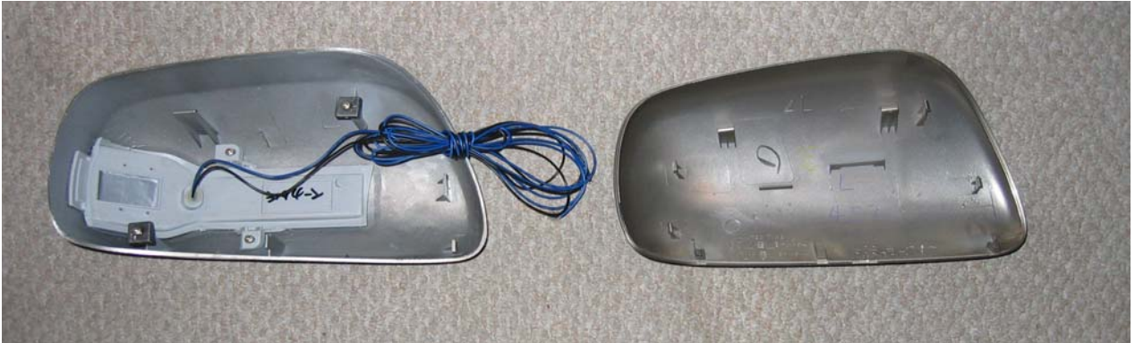
A side by side comparison of the LED turn signal mirror cover (left) with the OEM mirror cover (right).
