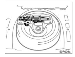
To remove the jack, unlock the tightening strap.
