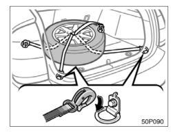
Attach the other ends of the belts to the rear tie-down hooks.
