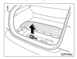
1. Remove the towing eyelet as shown in the illustration.
