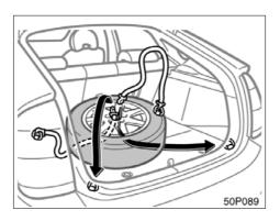
3. Pass the belts through the center hole of the wheel as shown above.
