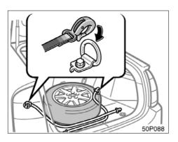
2. Put the flat tire on the center of the luggage storage box lid with the outer side of the wheel facing up. Hook one ends of the belts to the front tie-down hooks.
