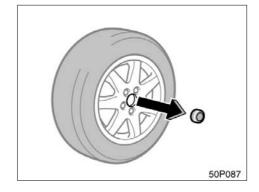
1. Before stowing the flat tire, remove the center wheel ornament by pushing from the reverse side.
