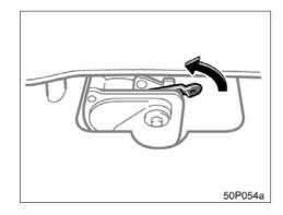
2. Pull the lever with the back door motor, open the back door.
