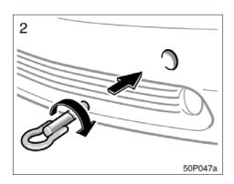
2. Secure the towing eyelet to the hole on the bumper by turning it clockwise.
