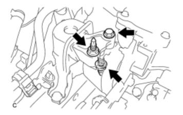
(c) Remove the bolt and 2 nuts, and separate the engine mounting insulator RH.
