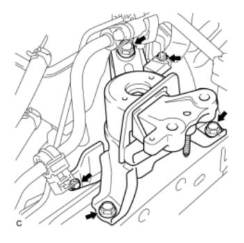
(a) Remove the 3 bolts and 2 cooler brackets.
