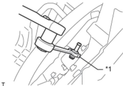
(b) Using a ball joint lock nut wrench (22 mm), remove the ventilation valve sub-assembly.
