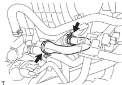
(a) Remove the ventilation hose from the ventilation valve sub-assembly.
