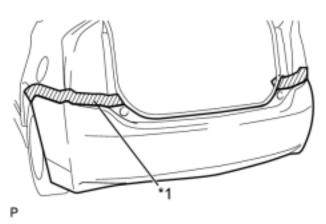
(a) Put protective tape around the rear bumper assembly.
