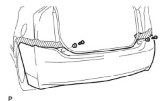
(b) Remove the 2 screws and 2 rear bumper upper stoppers.
