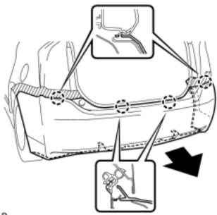
(h) Disengage the 4 claws and remove the rear bumper assembly as shown in the illustration.
