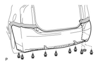
(c) Using a clip remover, remove the 9 clips.
