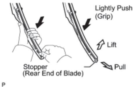
(a) Lift and pull the end of the wiper rubber protrusion from the blade stopper as shown in the illustration.
