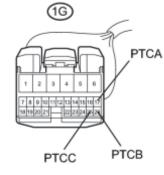
(b) Disconnect the engine room relay block and junction block (integration relay) connector.
