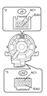
(a) Disconnect the connector from the spiral with sensor cable subassembly.
