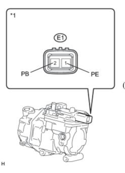
(f) Disconnect the connector from the compressor with motor assembly.
