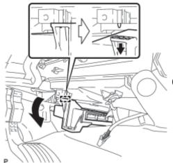
(b) Disengage the guide as shown in the illustration.
