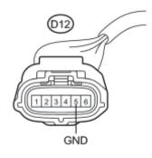
(a) Disconnect the connector from the compressor with motor assembly.
