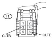
(a) Disconnect the solar sensor (automatic light control sensor) connector.
