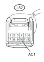
(a) Disconnect the connector from the spiral with sensor cable subassembly.
