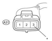
(a) Disconnect the A/C pressure sensor connector.
