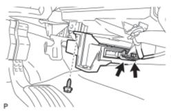
(a) Disconnect each connector and remove the screw.
