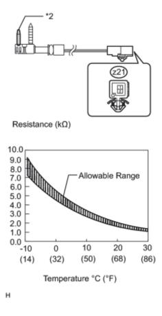
(c) Measure the resistance according to the value(s) in the table below.
