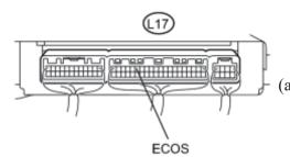
(a) Remove the A/C amplifier with the connectors still connected.
