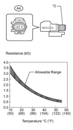
(c) Measure the resistance according to the value(s) in the table below.
