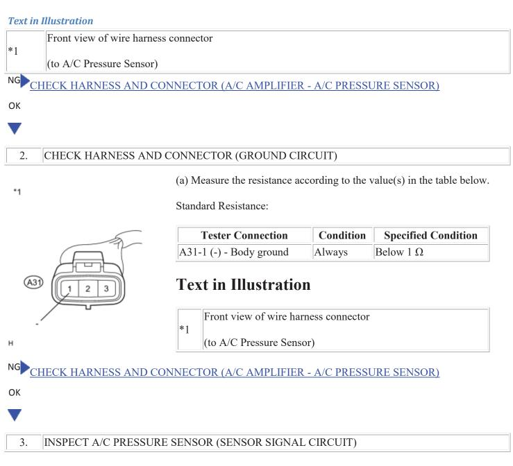
(a) Reconnect the A/C pressure sensor connector.
