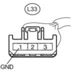
(a) Disconnect the blower motor connector.
