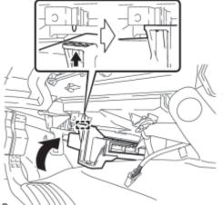
(b) Engage the guide and install the air conditioning amplifier assembly as shown in the illustration.
