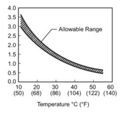
(c) Measure the resistance according to the value(s) in the table below.
