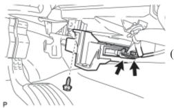
(c) Install the screw and connect each connector.
