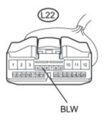
(b) Disconnect the solar ventilation ECU connector.
