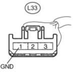
(a) Disconnect the blower motor connector.
