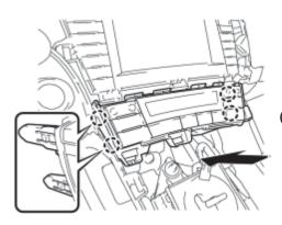
(b) Engage the 4 claws to install the air conditioning control assembly.
