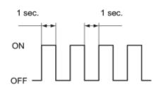
(d) The indicator check is automatically performed when panel diagnosis is activated. Check that the indicators light up and go off 4 times at 1-second intervals continuously.
