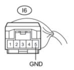
(a) Disconnect the plasmacluster (ion generator) connector.
