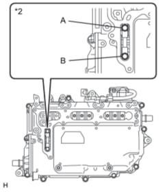
(d) Check that bolts A and B are tightened securely.
