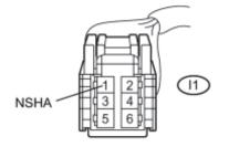
(a) Disconnect the solar sensor (automatic light control sensor) connector.
