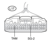
(a) Disconnect the A/C amplifier connector.
