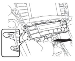
(a) Disengage the 4 claws and remove the air conditioning control assembly as shown in the illustration.
