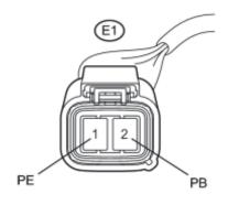
(a) Disconnect the No. 2 engine wire connector.
