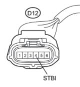
(b) Disconnect the connector from the compressor with motor assembly.
