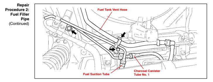
B. Disconnect the fuel tank vent hose (fuel tank side) from the clamp.
