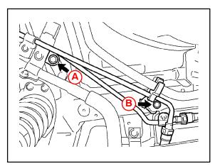
Repair Procedure 2: Fuel Filler Pipe (Continued) C. Install the fuel tube connector and fuel filler pipe clamp to the fuel tank inlet pipe.
