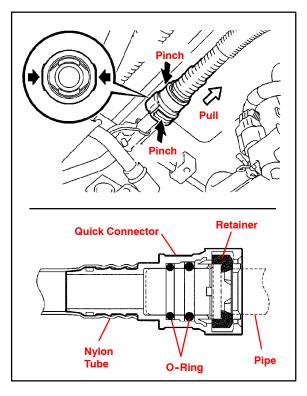
E. Remove the fuel filler pipe clamp and fuel tube connector from the fuel tank inlet pipe.
