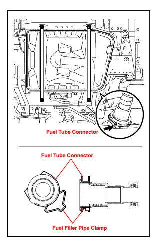
Repair Procedure 2: Fuel Filler Pipe (Continued) F. Remove the 2 bolts, then remove the fuel tank filler pipe sub-assembly.
