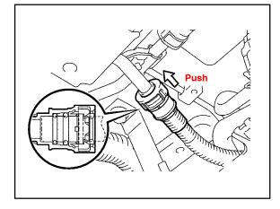
F. Install the fuel tank vent hose (fuel tank side) to the clamp.
