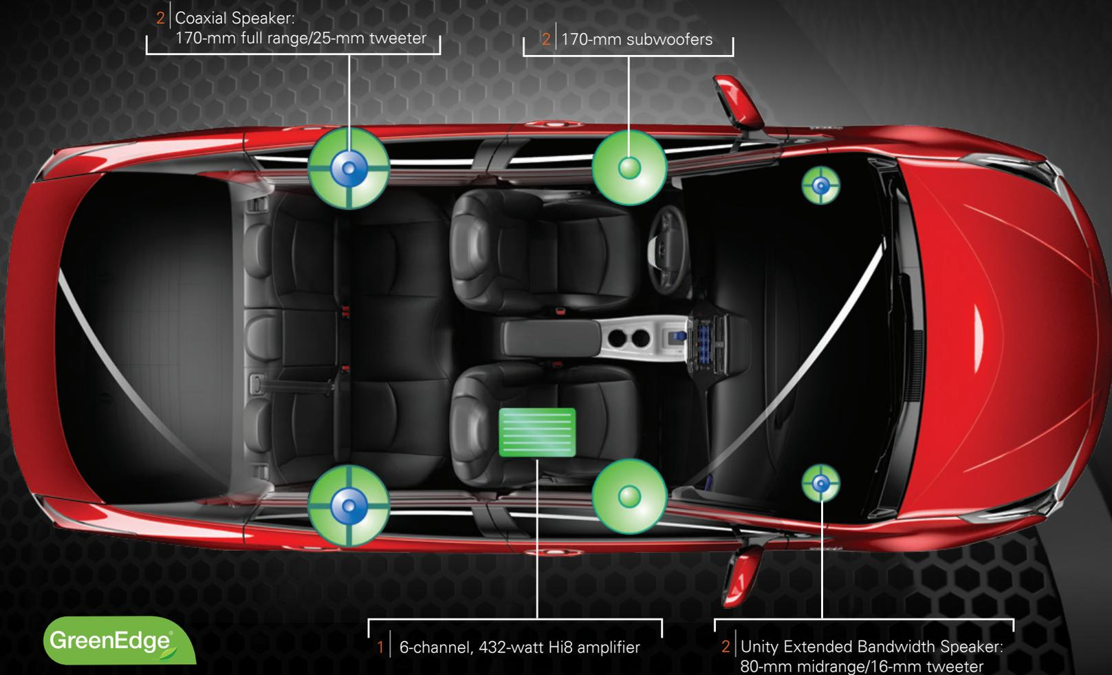
10 SPEAKERS IN 6 LOCATIONS, 432 WATTS, 6-CHANNEL, Hi8 AMPLIFIER
