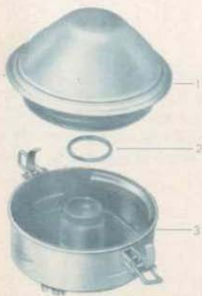
1-Filter element, 2-Gasket, 3-Oil reservoir
