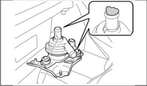
e) Plug the HV water pump ports with paper towels or shop cloths.
