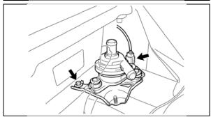
d) Reinstall the bolt and torque to spec.
