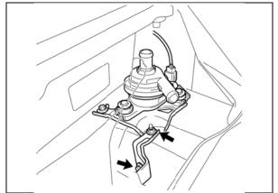
f) Reinstall the bracket with the bolt and nut, then torque to spec.
