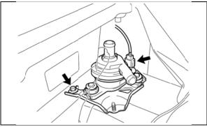
d) Remove the connector and bolt.
