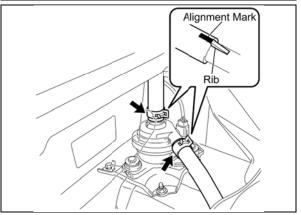
g) Using the alignment marks, reconnect the 2 hoses with the 2 clamps.
