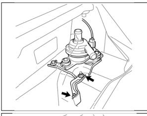
c) Remove the nut, bolt, and bracket.
