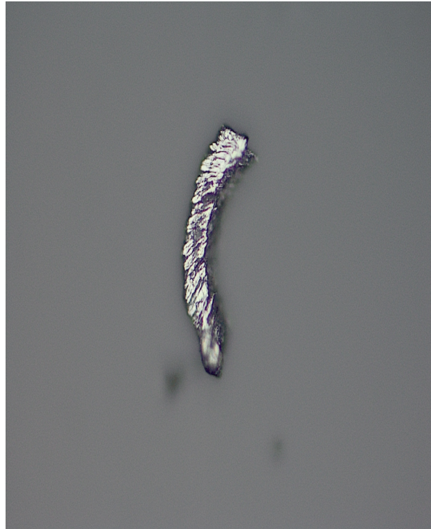
Figure 2: Large Ferrous Cutting Wear Particle and Abrasive/Dust/Dirt Particles at the Middle of the Slide (Magnification 500X).
