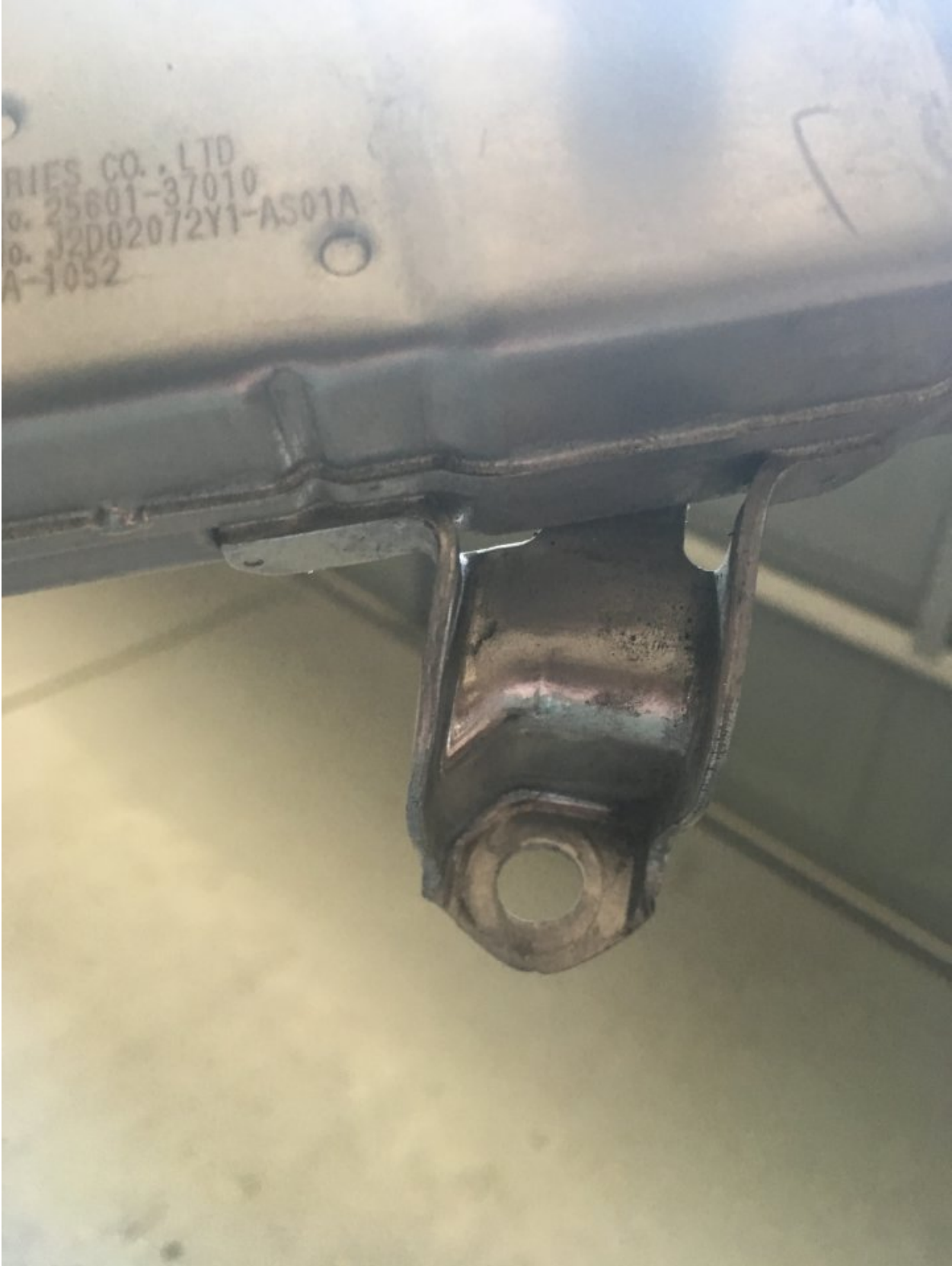
Figure 5 Bottom cooler support that I trimmed the bottom 2/3s of to aid in reassembly:
