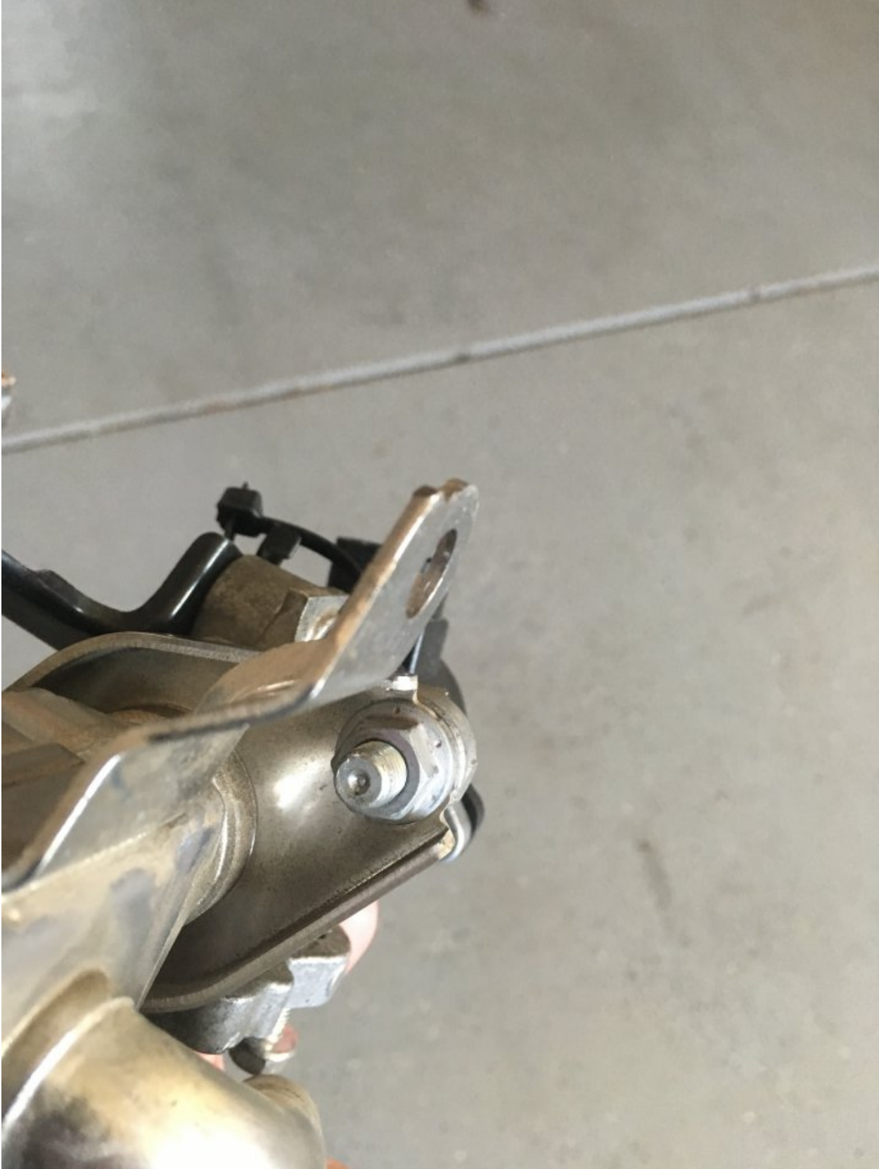
Figure 4 Left side of the from behind the egr valve looking at the 12mm nut:
