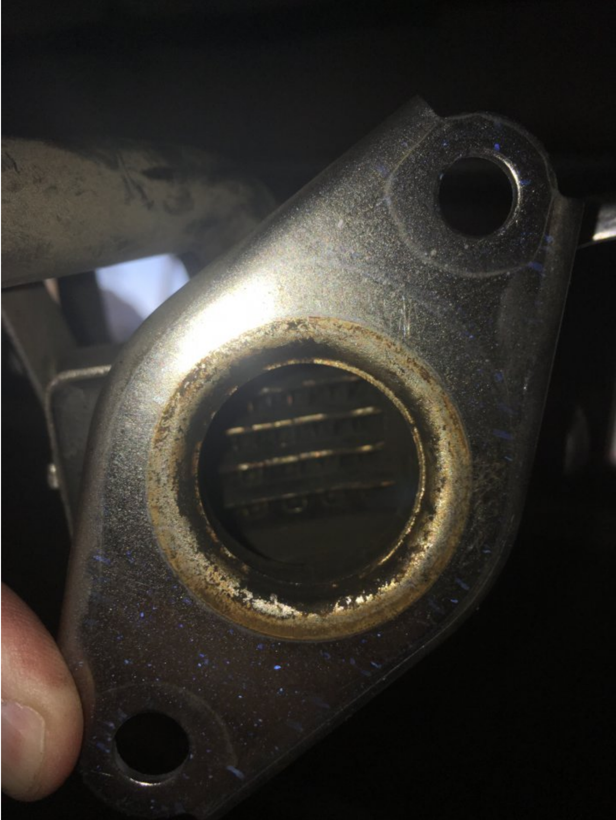
Figure 9 A look at the fins inside the egr cooler:
