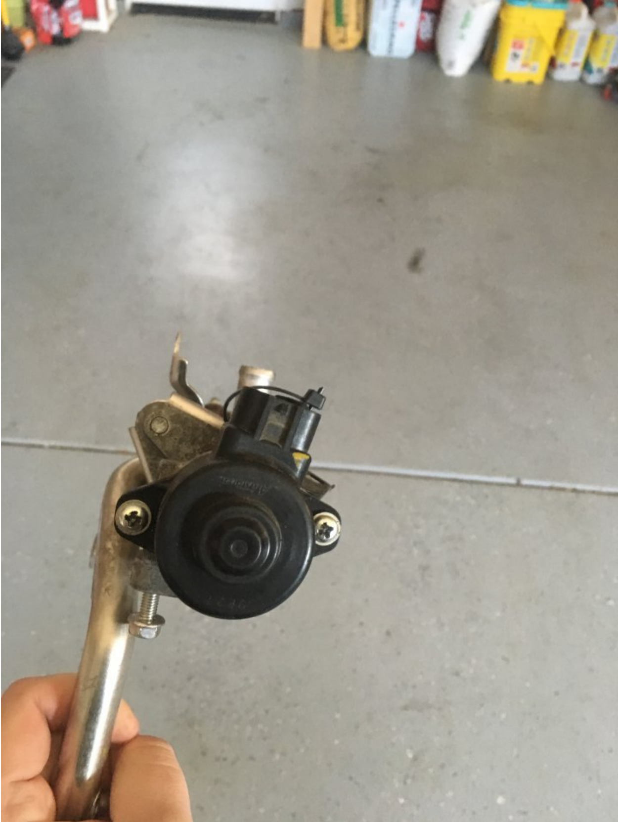
Figure 2 Egr valve from the top view that you can see from the engine bay:
