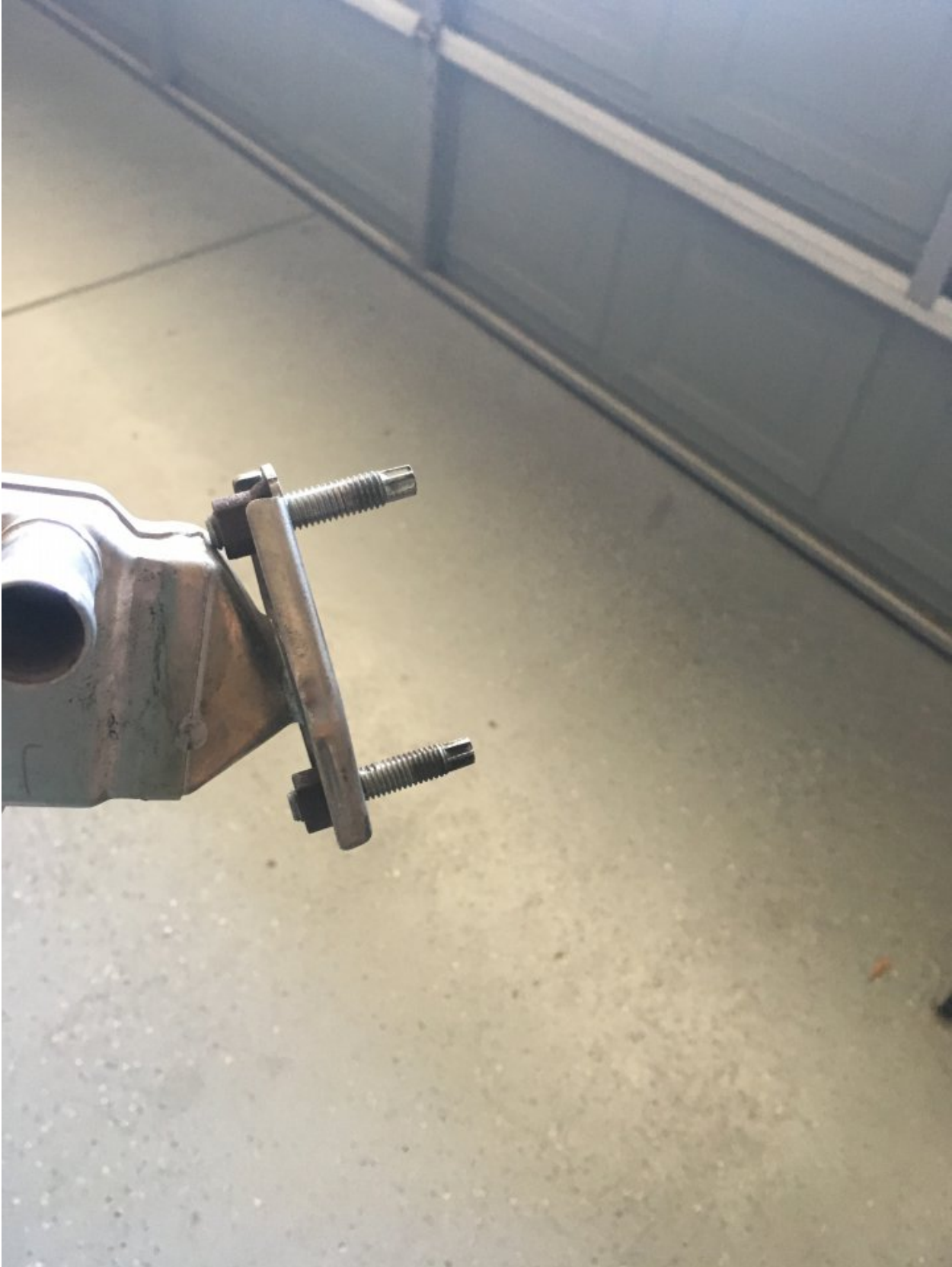
Figure 6 View of the back support studs for the cooler:
