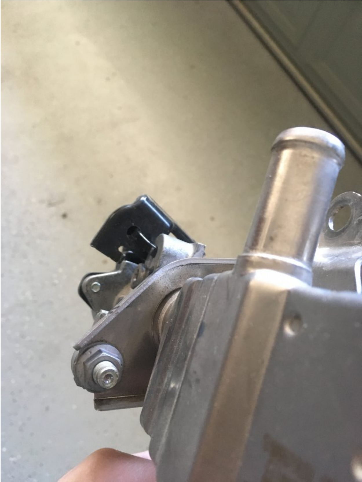
Figure 3 Right side from behind the egr valve looking at the 12mm nut that holds the egr valve to the cooler:
