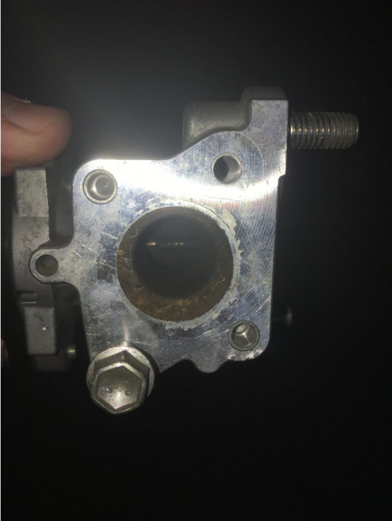
Figure 7 Downstream view of the egr valve (after the plunger of the egr where the egr pipes connect):
