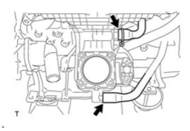
Disconnect the fuel vapor feed hose and ventilation hose.
