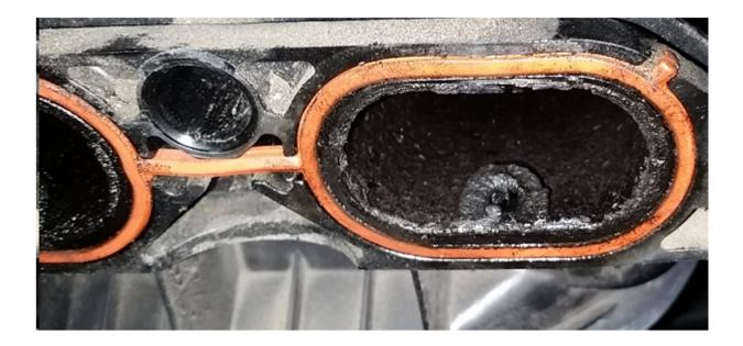
Carbon deposits clogging intake manifold (Prius.2)
