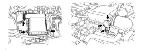
Air Filter Cap + Mass Air Flow Connector
