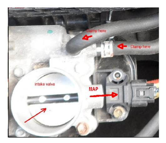
Clamp off Coolant Hoses before removing from the throttle body.
