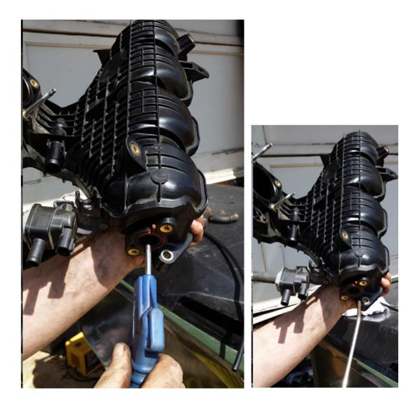
Cleaning Carbon Deposits with Air Nozzle
