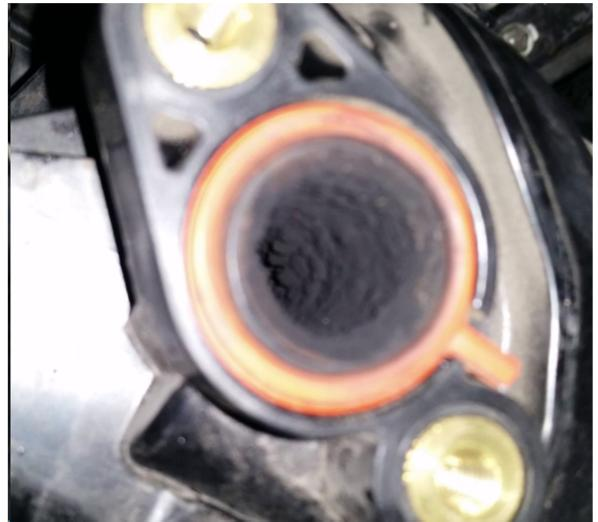
Carbon Deposits in the Intake Manifold EGR Inlet – Dryer / Sootier deposits (Prius.2)
