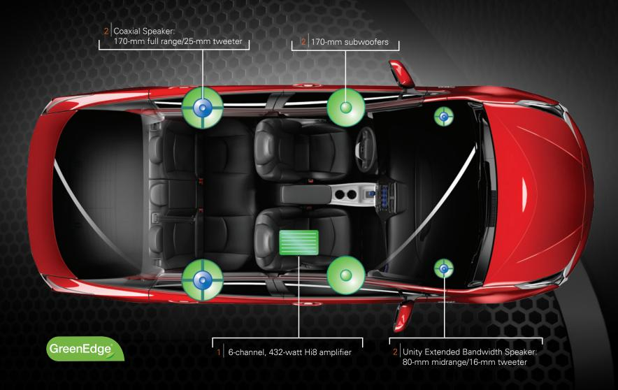
10 SPEAKERS IN 6 LOCATIONS, 432 WATTS, 6-CHANNEL, Hi8 AMPLIFIER
