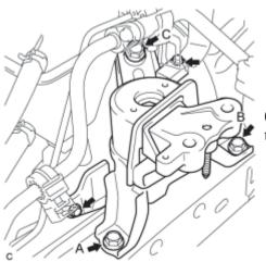
(a) Position the engine mounting insulator sub-assembly RH as shown in the illustration.
