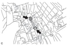
(d) Remove the bolt and nut, and separate the engine mounting insulator LH.
