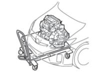
(c) Set the engine assembly with transaxle and front suspension crossmember on the engine lifter.
