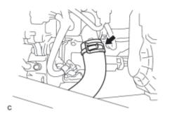
(a) Disconnect the No. 2 radiator hose from the water inlet.
