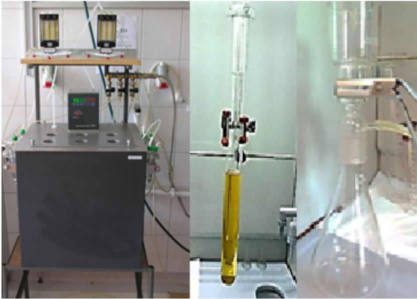
Figure 27. A test assembly for oxidation-stability tests of diesel fuels according to the standard EN 12205.
