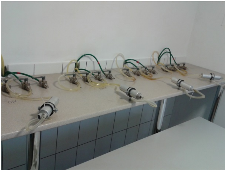
Figure 18. Liquid fuel sampling station.
