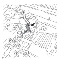
(a) Sufficiently apply compressor oil to a new air conditioning pressure sensor.
