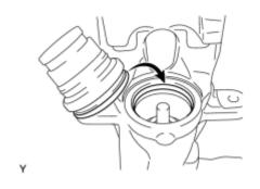
(a) Install the seal portion of the cylinder boot into the groove portion of the rear disc brake cylinder assembly.
