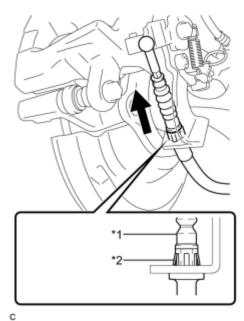
(a) Install the No. 3 parking brake cable assembly to the rear disc brake cylinder assembly.
