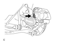
(a) Connect the front flexible hose to the disc brake cylinder assembly with a new union bolt and a new gasket.
