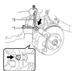
(a) Hold the front disc brake cylinder slide pin, and install the disc brake cylinder assembly to the front disc brake cylinder mounting with the 2 bolts.
