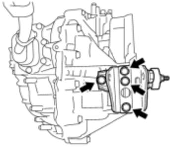
14. REMOVE ENGINE MOUNTING BRACKET LH
