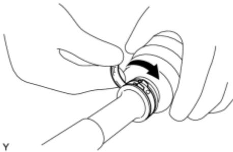
(a) Install the front axle outboard joint boot clamp onto the outboard joint boot and temporarily fold back the lever.
