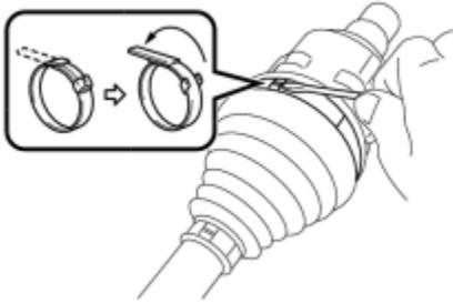
(a) Using a screwdriver, release the staked part of the front No. 2 axle inboard joint boot clamp and separate the front No. 2 axle inboard joint boot clamp as shown in the illustration.
