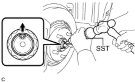
(a) Using SST and a hammer, release the staked part of the front axle shaft nut.
