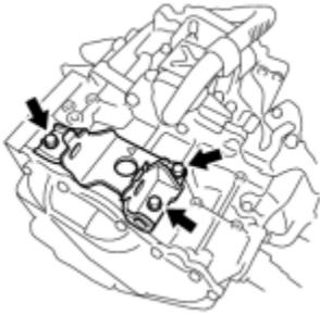
(a) Remove the 3 bolts and engine mounting bracket LH.
