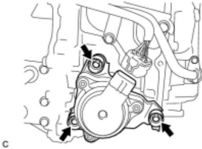
(a) Install the shift control actuator assembly with the 3 new shift control actuator bolts.
