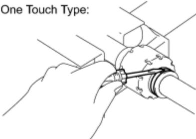
(1) Using a screwdriver, install a new front drive shaft damper clamp, as shown in the illustration.
