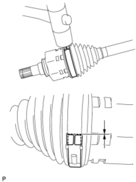
(f) Using a plastic hammer, tap the buckle to secure it while adjusting the clearance between the lever and the groove to make the clearance between the buckle edge and the lever end even.
