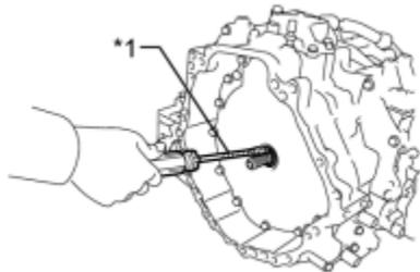
(a) Using a screwdriver with the tip taped, remove the oil seal.
