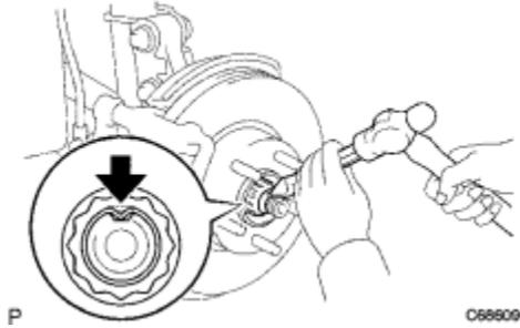
(a) Using a chisel and hammer, stake the front axle shaft nut.
