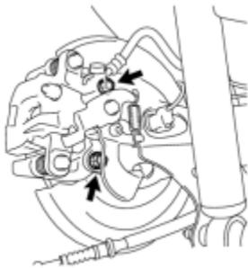
(a) Install the rear disc brake caliper assembly with the 2 bolts.
