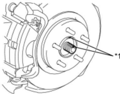
(b) Align the matchmarks and install the front drive shaft assembly to the front axle hub sub-assembly.
