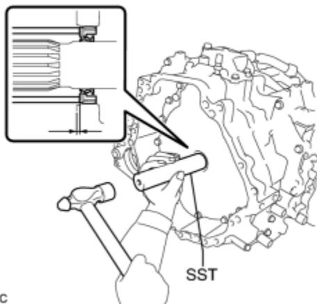
(a) Coat a lip of a new oil seal with MP grease.
