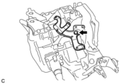
(a) Remove the bolt and motor cable bracket.
