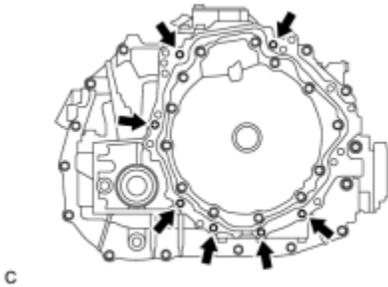
(b) Remove the 7 bolts and hybrid vehicle transaxle assembly.
