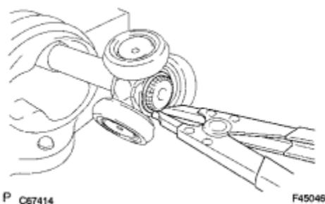
(f) Using a snap ring expander, install a new shaft snap ring to the front axle outboard joint shaft assembly.
