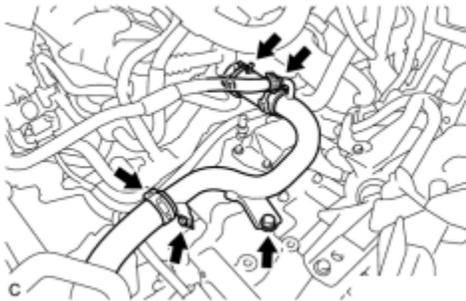
(a) Disconnect the clamps, No. 1 radiator hose, No. 4 water by-pass hose and No. 3 radiator hose.
