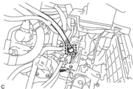
(a) Disconnect the generator cable clamp from the motor cable bracket.
