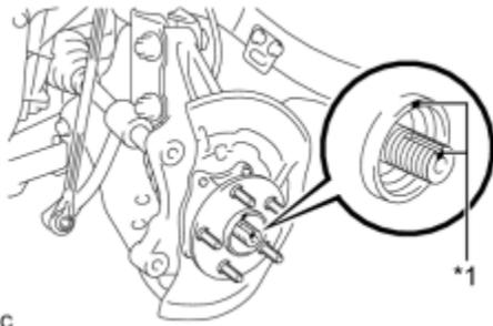
(a) Put matchmarks on the front drive shaft assembly and front axle hub sub-assembly.
