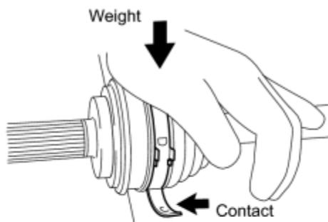
(b) Lean your weight on your hand and roll the outboard joint forward while pressing the outboard joint against the work plane. Roll the outboard joint and fold the lever until a click sound can be heard.
