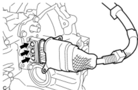
(d) Remove the 3 bolts and motor cable from the hybrid transaxle assembly.
