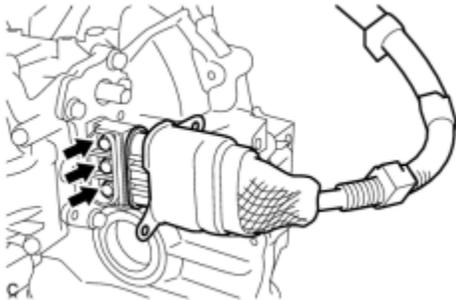
(a) Install the motor cable to the hybrid transaxle assembly with the 3 bolts.
