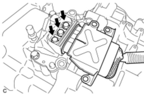
(a) Install the generator cable to the hybrid transaxle assembly with the 3 bolts.
