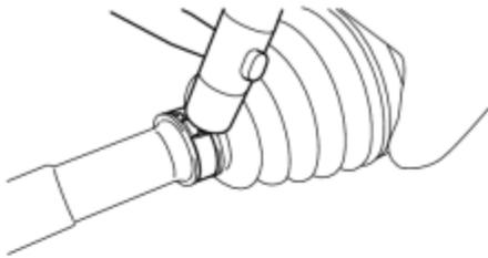
(c) Using a plastic hammer, tap the buckle to secure it while adjusting the clearance between the lever and the groove to make the clearance between the buckle edge and the lever end even.
