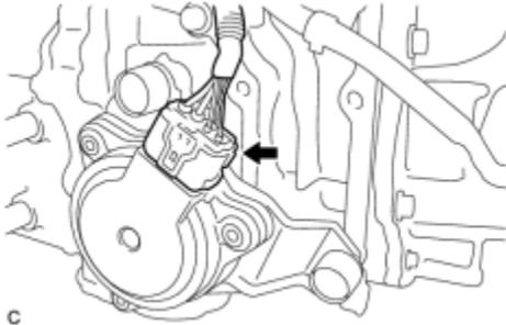
(a) Disconnect the connector from the shift control actuator assembly.
