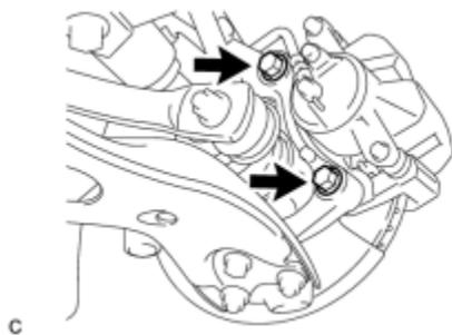
(a) Remove the 2 bolts and separate the front disc brake caliper assembly.
