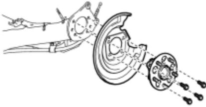
(a) Install the rear axle hub and bearing assembly and rear disc brake dust cover to the rear axle beam assembly with the 4 bolts.
