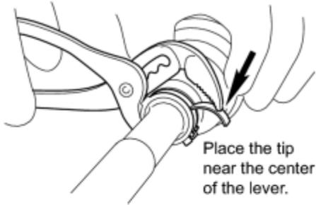
(b) Using water pump pliers, pinch the front axle outboard joint boot clamp to temporarily secure it.
