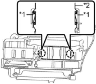
(a) Engage the 2 claws to install the transmission control ECU assembly to the ECU integration box.
