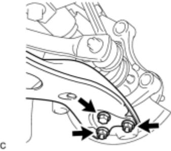
(a) Install the front No. 1 lower suspension arm sub-assembly to the front lower ball joint with the bolt and 2 nuts.
