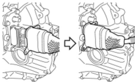
(c) Place the motor cable connector shell in position and install it with the 2 bolts.
