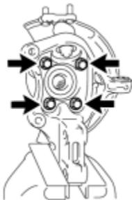
(b) Remove the 4 bolts, front axle hub sub-assembly and front disc brake dust cover.
