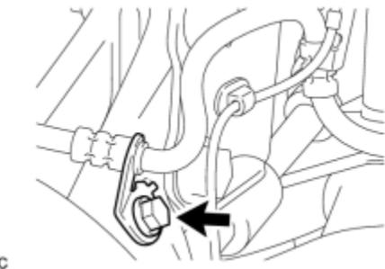
(a) Remove the bolt and separate the front flexible hose from the steering knuckle.
