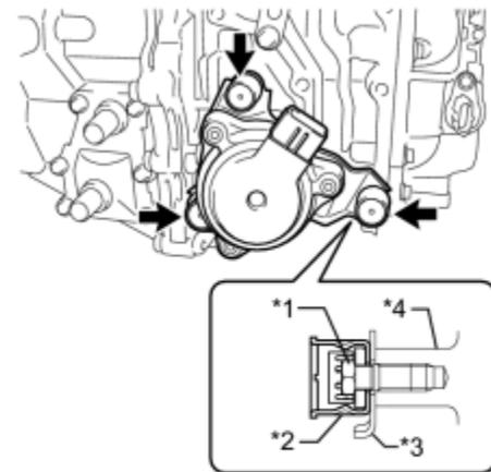
(b) Using pliers or an equivalent tool, turn the shift control actuator bolt covers counterclockwise and remove the 3 shift control actuator bolts and shift control actuator assembly.
