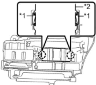
(a) Disengage the 2 claws and remove the transmission control ECU assembly from the ECU integration box.
