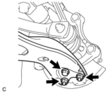
(a) Remove the bolt and 2 nuts, and separate the front No. 1 lower suspension arm sub-assembly from the front lower ball joint.
