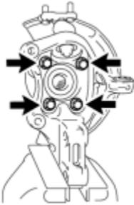
(b) Install the front axle hub sub-assembly and front disc brake dust cover with the 4 bolts.
