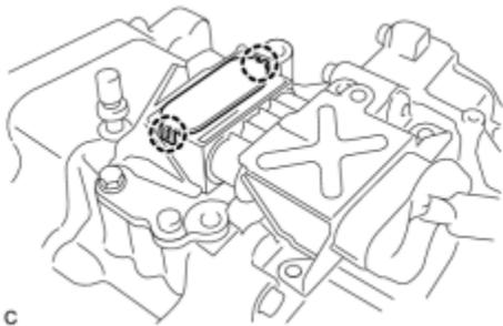
(b) Engage the 2 claws to install a new terminal cap.
