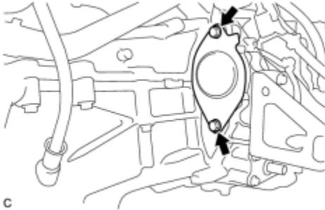
(a) Install the starter hole insulator with the 2 bolts.
