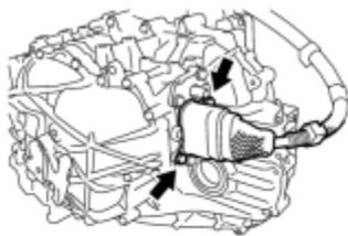
(b) Remove the 2 bolts and slide the motor cable connector shell back.
