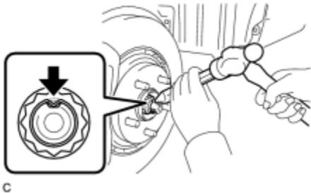
(b) Using a socket wrench (30 mm), install the axle shaft nut.
