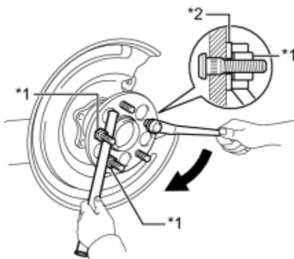
(a) Temporarily install a new rear axle hub bolt to the rear axle hub and bearing assembly.
