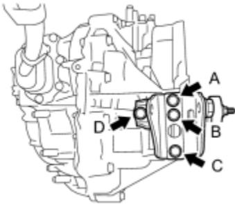
(a) Install the rear engine mounting bracket with the 4 bolts in several steps.
