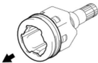
(i) Remove the front axle inboard joint grommet from the front drive inboard joint assembly.
