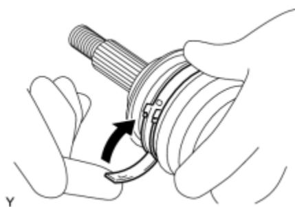
(a) Install the front No. 2 axle outboard joint boot clamp onto the outboard joint boot and temporarily fold back the lever.
