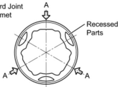
(c) While keeping dimension (A) within the specified length, put the inside of the inboard joint under atmospheric pressure by pulling the recessed parts on the inboard joint grommet out.
