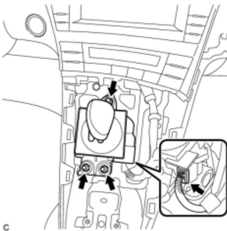
(a) Disconnect the connector from the shift lock control unit assembly.
