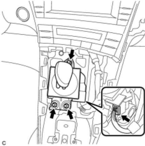
(a) Install the shift lock control unit assembly with the 3 nuts.
