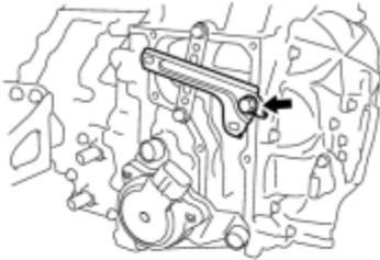
(a) Install the 2 wire harness clamp brackets with the 2 bolts.
