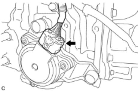
(c) Connect the connector to the shift control actuator assembly.
