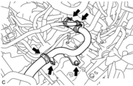
(a) Install the radiator pipe with the 2 bolts.
