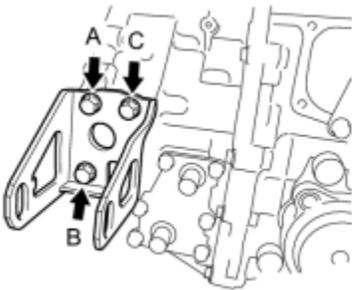
(a) Install the front engine mounting bracket with the 3 bolts in several steps.
