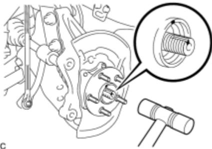
(b) Using a plastic hammer, separate the front drive shaft assembly from the front axle assembly. If it is difficult to separate, tap the end of the front drive shaft assembly using a brass bar and a hammer.
