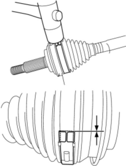
**5. INSTALL FRONT AXLE OUTBOARD JOINT BOOT CLAMP (for LH Side)**
