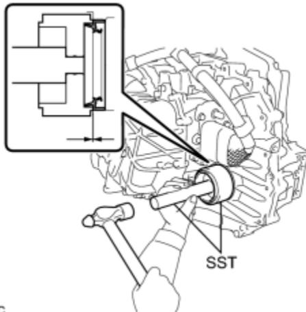
(1) Using SST and a hammer, tap in a new oil seal.
