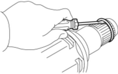
(a) Using a screwdriver, remove the front drive shaft hole snap ring.
