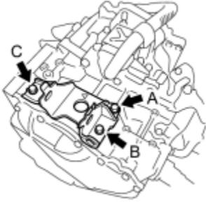
(a) Install the engine mounting bracket LH with 3 new bolts in several steps.
