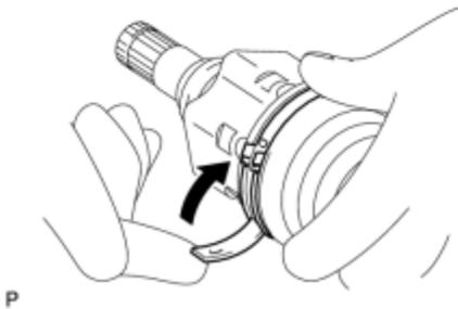
(d) Set the lever fulcrum point at any point A indicated in the illustration and temporarily bend the lever.
