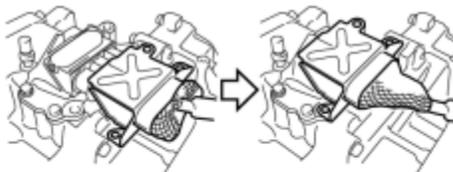
(c) Place the generator cable connector shell in position and install it with the 3 bolts.
