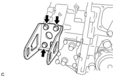
(a) Remove the 3 bolts and front engine mounting bracket.
