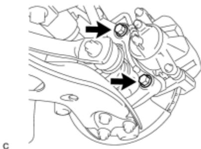
(a) Install the front disc brake caliper assembly to the steering knuckle with the 2 bolts.
