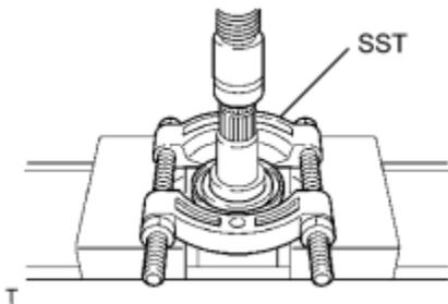
(a) Using SST and a press, remove the front drive shaft dust cover from the front drive inboard joint assembly.
