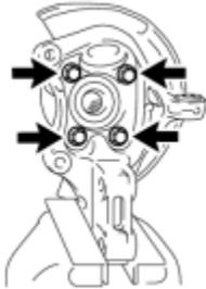
(b) Install the front axle hub sub-assembly and front disc brake dust cover with the 4 bolts.
