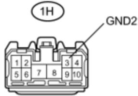
(c) Connect the integration relay connectors.
