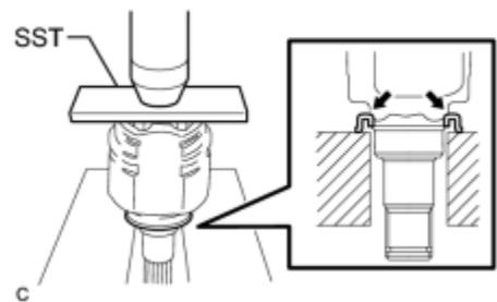
(a) Using SST and a press, install a new front drive shaft dust cover into the front drive inboard joint assembly until it is flush with the end.
