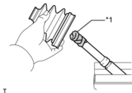
(a) Wrap the splines of the front axle outboard joint shaft assembly with protective tape to prevent the boot from being damaged.
