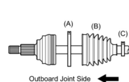
(b) Install new parts onto the front axle outboard joint shaft assembly in the following order:
