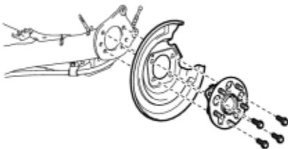
(a) Remove the 4 bolts, rear axle hub and bearing assembly and rear disc brake dust cover from the rear axle beam assembly.
