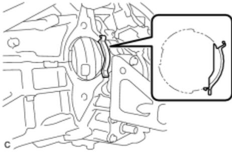
(a) Remove the flywheel housing side cover.
