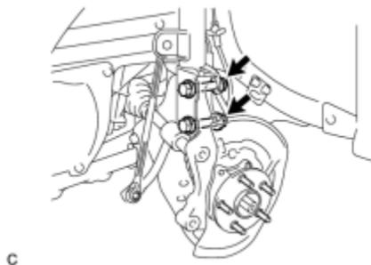
(a) Remove the 2 bolts, 2 nuts and front axle assembly.
