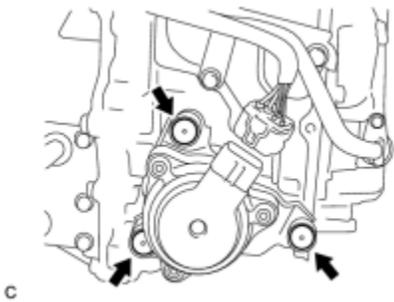
(b) Install the 3 new shift control actuator bolt caps to the shift control actuator bolts.
