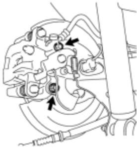
(a) Remove the 2 bolts, and separate the rear disc brake caliper assembly.
