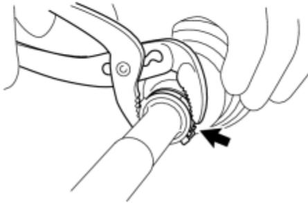
(c) Using a plastic hammer, tap the buckle to secure it while adjusting the clearance between the lever and the groove to make the clearance between the buckle edge and the lever end even.
