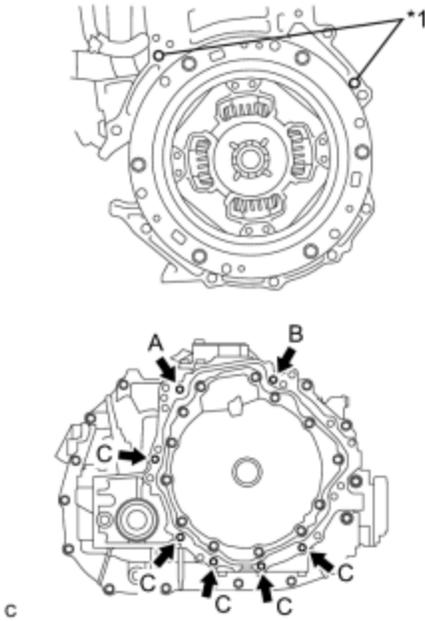
(b) Using an engine lifter, align the engine assembly and hybrid vehicle transaxle assembly, fit the knock pins into the knock pin holes, and tighten the 7 bolts shown in the illustration.
