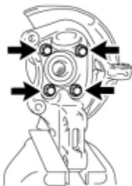
(b) Remove the 4 bolts, front axle hub sub-assembly and front disc brake dust cover.
