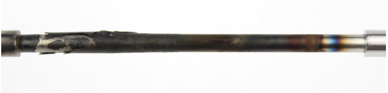
Figure 47: Conventional oil #2 TEOST 33C rod deposits
