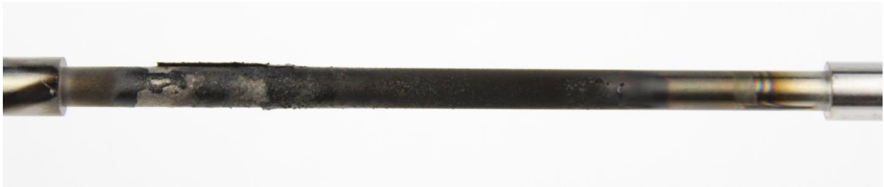
Figure 63: Synthetic oil #5 TEOST 33C rod deposits
