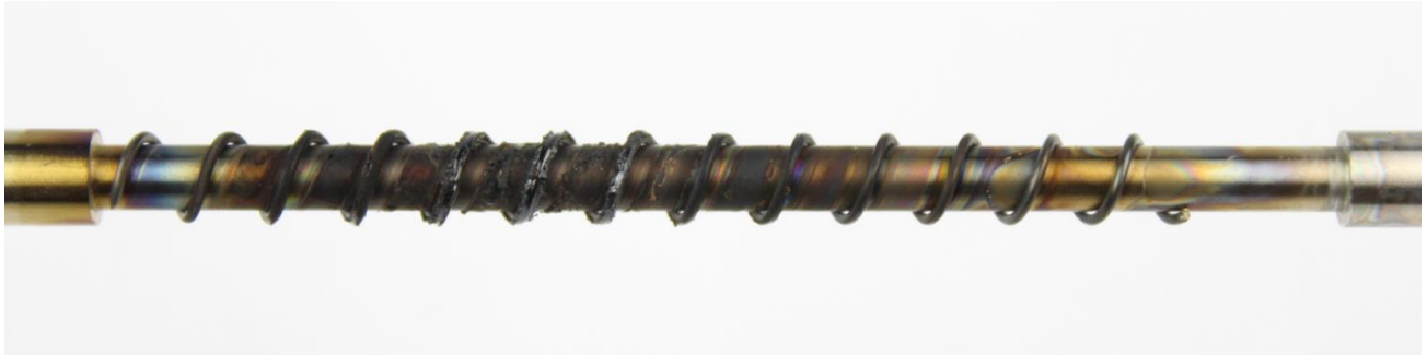
Figure 50: Conventional oil #4 TEOST MHT rod deposits
