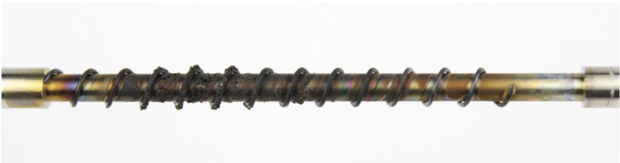
Figure 52: Conventional oil #5 TEOST MHT rod deposits
