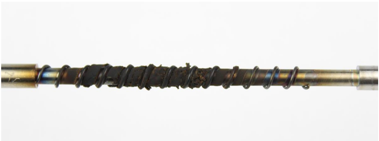
Figure 46: Conventional oil #2 TEOST MHT rod deposits
