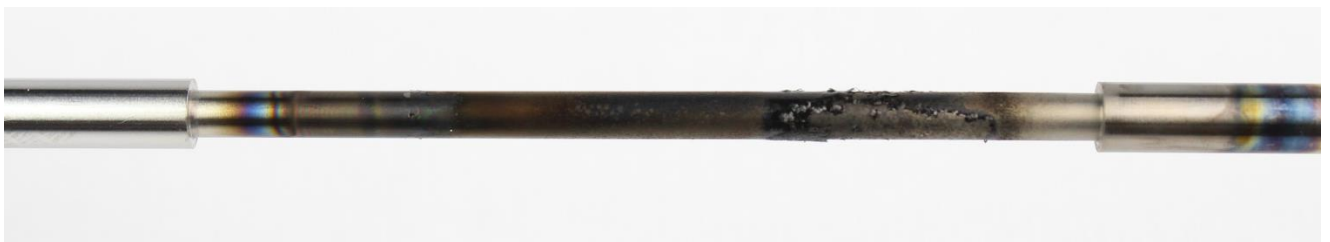
Figure 57: Synthetic oil #2 TEOST 33C rod deposits
