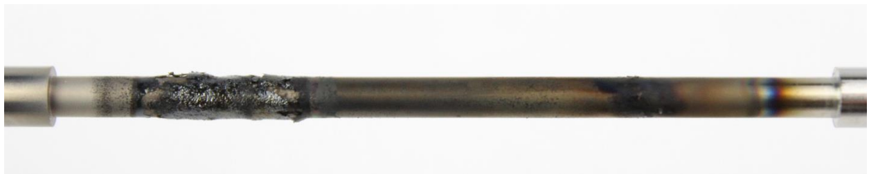
Figure 61: Synthetic oil #4 TEOST 33C rod deposits
