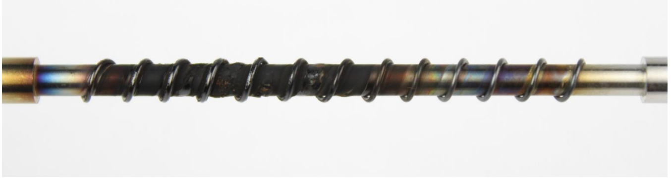
Figure 54: Synthetic oil #1 TEOST MHT rod deposits
