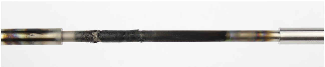
Figure 45: Conventional oil #1 TEOST 33C rod deposits
