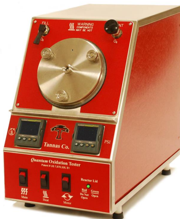
Figure 22: ASTM D4742 TFOUT instrument Image Source: AAA
