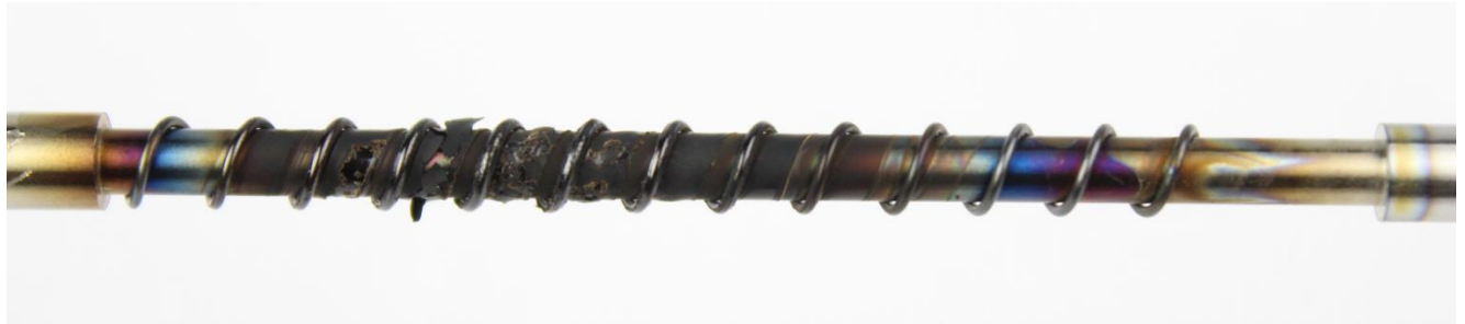
Figure 58: Synthetic oil #3 TEOST MHT rod deposits
