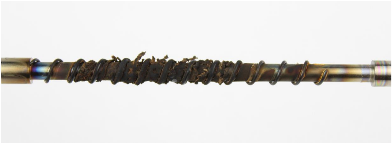
Figure 48: Conventional oil #3 TEOST MHT rod deposits
