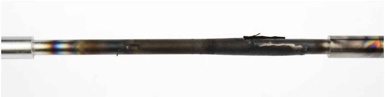
Figure 49: Conventional oil #3 TEOST 33C rod deposits
