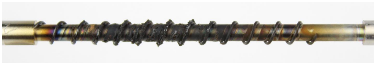
Figure 60: Synthetic oil #4 TEOST MHT rod deposits
