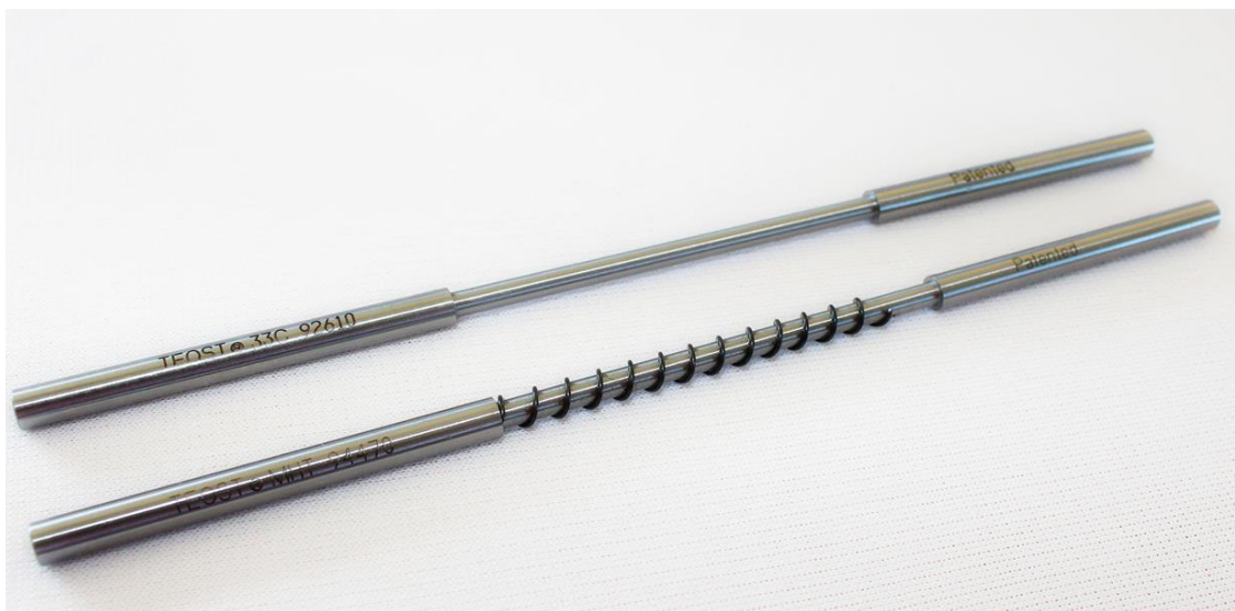
Figure 43: TEOST MHT & 33C depositor rods
