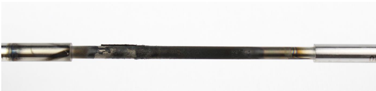
Figure 53: Conventional oil #5 TEOST 33C rod deposits
