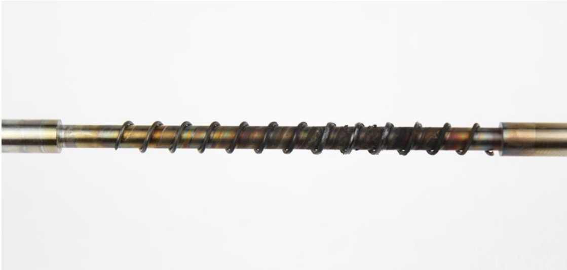
Figure 44: Conventional oil #1 TEOST MHT rod deposits
