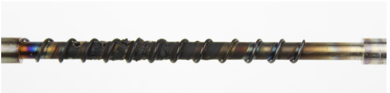
Figure 56: Synthetic oil #2 TEOST MHT rod deposits
