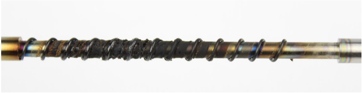
Figure 62: Synthetic oil #5 TEOST MHT rod deposits
