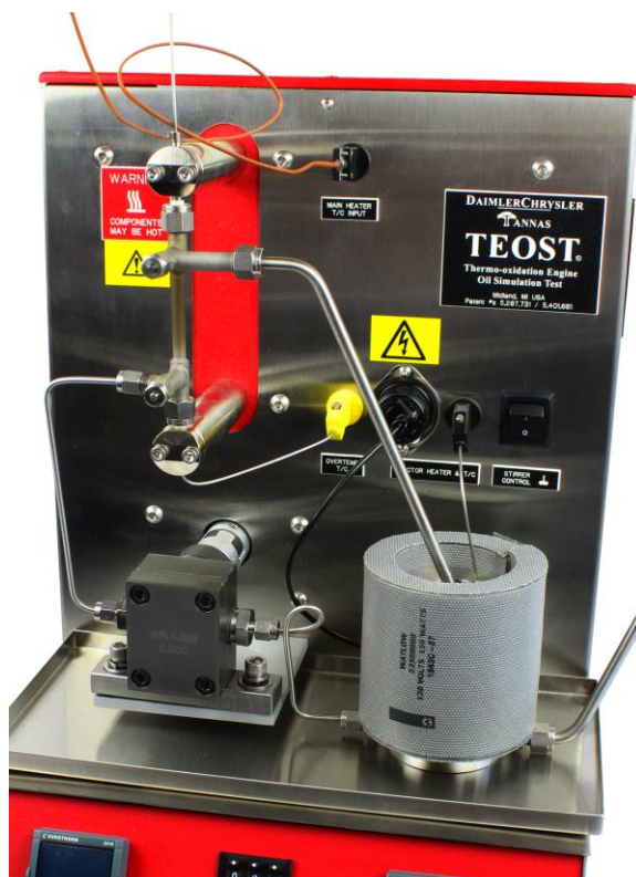
Figure 12: ASTM D6335 TEOST 33C instrument Image Source: AAA
