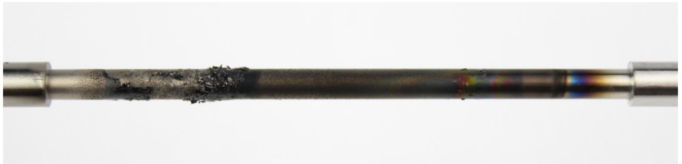
Figure 59: Synthetic oil #3 TEOST 33C rod deposits
