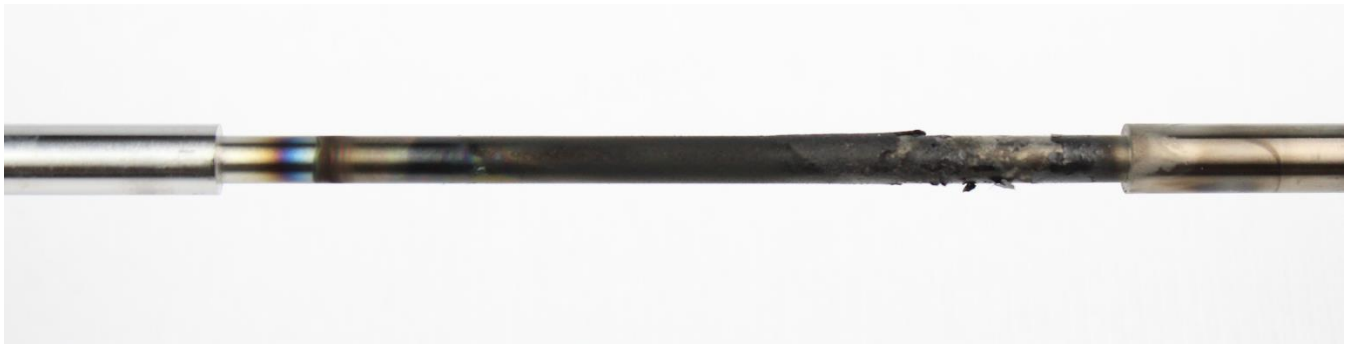
Figure 55: Synthetic oil #1 TEOST 33C rod deposits
