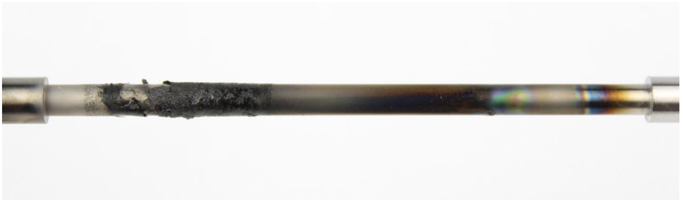
Figure 51: Conventional oil #4 TEOST 33C rod deposits
