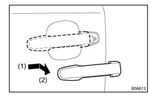
(b) Pushing and pulling the outside handle in the arrow mark direction as shown in the illustration, remove the outside handle.
