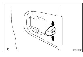
(c) Using pliers, remove the clip and handle frame, as shown in the illustration.
