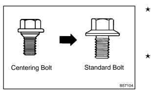
Centering bolts are used to mount the hood hinge and hood lock. The hood and hood lock cannot be adjusted with the centering bolts on. Substitute the centering bolts with standard bolts (w/ washers) when making adjustments.
