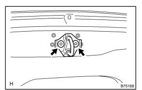
(b) Using a torx wrench (T40), remove the 2 screws and striker.
