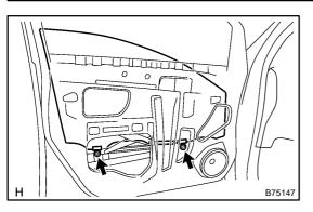
Install the door glass to the window regulator with the 2 bolts.
