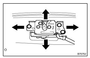
(c) Vertically adjust the rear end of the back door panel by loosening the back door lock bolts.
