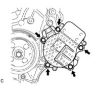
(b) Remove the 5 bolts and water pump assembly from the timing chain cover.
