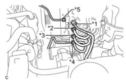
(c) Using a union nut wrench, disconnect the 5 brake lines from the brake booster with master cylinder assembly.
