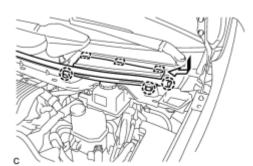
(1) Engage the 2 claws and 3 guides to install the center cowl top ventilator cover.
