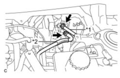
(a) Move the 2 clips and disconnect the No. 1 reservoir hose and No. 2 reservoir hose from the brake booster with master cylinder assembly.
