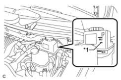
(a) Inspect the fluid level is above the MIN line with the power switch on (IG). If necessary, refill the brake fluid to the fluid level support line with the power switch on (IG).
