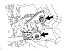
(a) Remove the 2 nuts and No. 5 brake actuator bracket.
