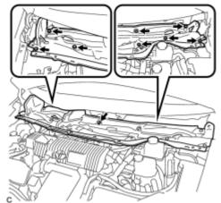
(a) Install the outer cowl top panel sub-assembly with the 9 bolts.
