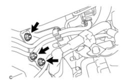
(f) Remove the 3 nuts and brake booster pump assembly with bracket.
