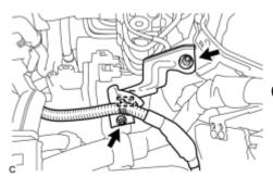
(a) Disengage the clamp.
