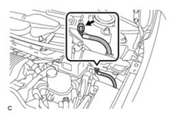
(b) Disconnect the reservoir level switch connector.
