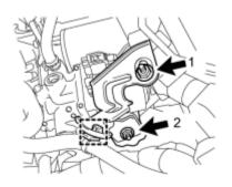
(a) Install the No. 5 brake actuator bracket with the 2 nuts.
