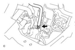
(a) Move the clip and disconnect the brake actuator hose from the brake booster pump assembly.
