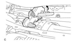
(b) Bend the water guard plate RH and engage the claw.
