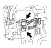
(a) Disconnect the 2 connectors and separate the clamp from the brake booster pump assembly.
