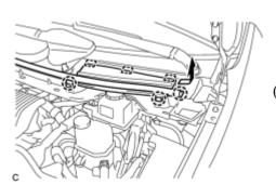
(1) Slide the hood to cowl top seal and disengage the claw.
