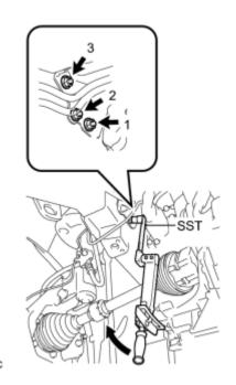
(b) Install the wire harness clamp, 2 fuel lines and front No. 4 brake tube to the brake booster pump assembly.
