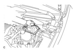
(1) Remove the brake master cylinder reservoir filler cap assembly.
