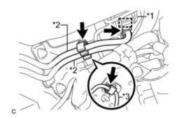
(e) Separate the wire harness clamp, 2 fuel lines and front No. 4 brake tube from the brake booster pump assembly.
