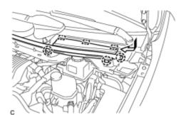
(1) Engage the 2 claws and 3 guides to install the center cowl top ventilator cover.
