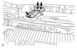
(a) Install the cowl body mounting reinforcement LH with the 3 bolts.
