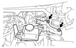
(a) Install the brake master cylinder reservoir with bracket with the 2 nuts.
