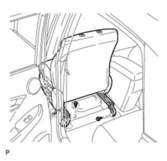
(a) Remove the 2 bolts on the rear side of the seat.
