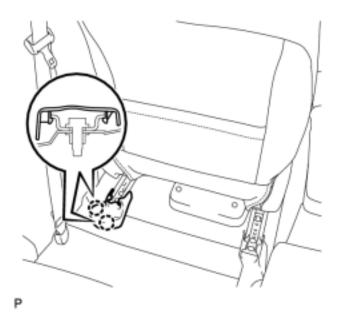
(a) Lift up the seat track adjusting handle and move the seat to the foremost position.
