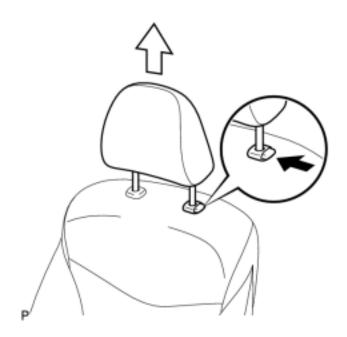
(a) Press the headrest support button and pull up the headrest as shown in the illustration to remove it.
