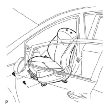
(c) Remove the 2 bolts on the front side of the seat.
